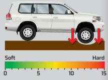
Rebound damping primarily affects vehicle traction, damper top-out and vehicle body movements such as vehicle pitch, dive and roll.
