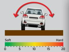
Low speed compression primarily affects the compression damping during low speed shaft movements such as vehicle pitch, dive and roll, wheel traction and vehicle ride (harshness and plushness).
