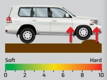
High speed Compression primarily affects the compression damping during high speed shaft movements such as harsh or square edge bumps and harsh vehicle landings.
