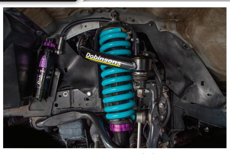
Built on the back of the race winning Monotube Remote Reservoir (MRR) shock absorbers, Dobinsons new range of MRR Adjustable shock absorbers combine the best in high performance race-bred Monotube technology, with an all new 3-way damping adjustment system to turn your 4x4 into the ultimate off-road machine. Each component of the MRR shock absorber has been refined and improved to offer a higher level of ride quality, vehicle control and shock absorber performance.
