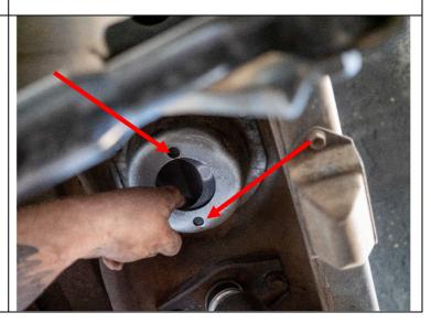
6. Bolt the bump stop and mount into the vehicle using the bolts supplied and red high strength Loctite using the M8 x 35mm bolts, spring washers and flat washers combined, bolting to he half circle plates. Bolt one side in first to hold the half circle plate and then rotate into place to get the second nut.
