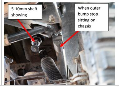
Tighten the lock nut on the hydraulic bump stop and then tighten the locking grub screw
