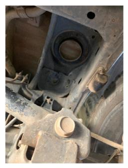
Dobinsons Springs and Suspension Hollingsworth Street Australia/USA/UAE 58 Hollingsworth Street NORTH ROCHAMPTON QLD AUSTRALIA <u>admin@dobinsonsprings.com</u> **5.** Refit the coil with the Hydraulic bump stop assembly mounted in the coil. If you have a different longer travel shocks read below notes before proceeding with this step.
