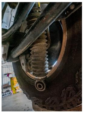
4. Lower the differential until the coil and OEM bump stop can be removed.
