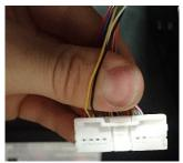
8. Strip the Yellow and Black wires in preparation for joining with the ARB harness.
