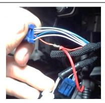
18. Cover exposed wire with electrical tape and bundle all wires with soft tape.
