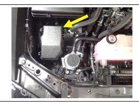
46. With 10mm socket, remove the three bolts securing the fuse box to the vehicle body.
