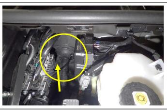
22. In preparation to bring Harness ® through the firewall, take the **Firewall Connector** and tape onto a plastic pipe as shown.
