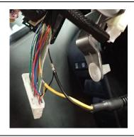
11. Cover exposed wires with electrical tape and bundle all wires with soft tape.
