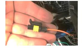
60. Join the **Fuse Box Connectors** together (plug connector and socket connector).
