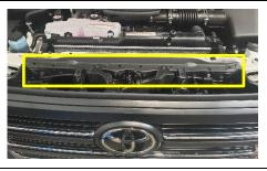
35. Find the **Ground Terminal** on Harness **(B)**. Fix the **Ground Terminal** onto a suitable grounding point on vehicle body or chassis.
