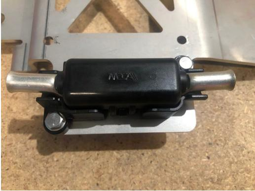
3. Remove original battery clamp from the main battery note: COLORADO, DMAX and MUX the battery clamp mounts to the top of the existing factory battery clamp
