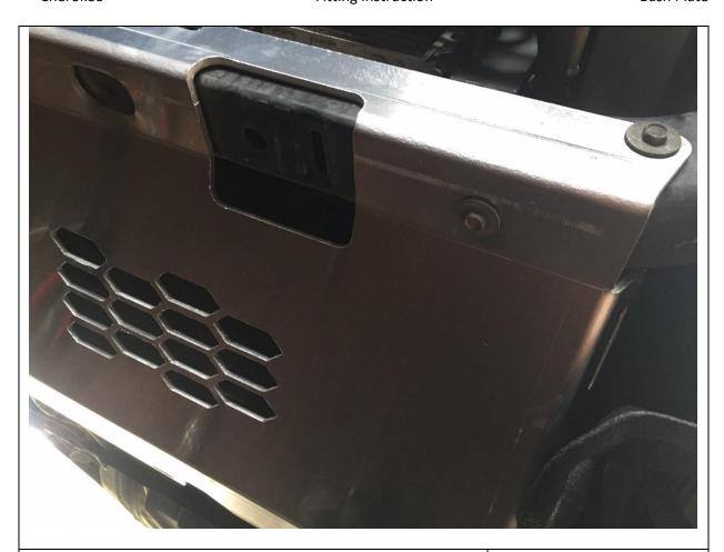
5. Reuse factory hardware and secure front of plate to cross member
