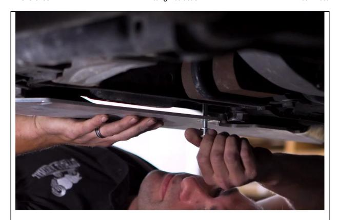
6. Fit M8 Button head cap screws to rear of bash plate in factory threaded clips
