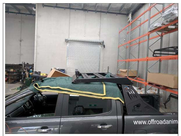
9. With Assistance, lift roof rack onto roof of vehicle. Place rear of rack assembly where roof rack bolts to sail.
