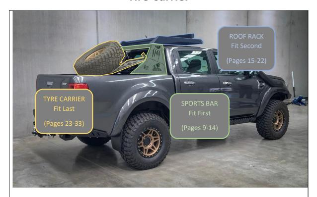
1. If fitting roof rack portion of chase rack do this before fitting tire carrier.
