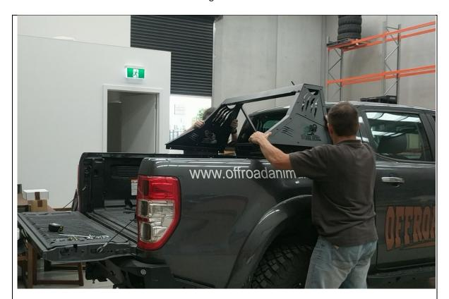
6. With assistance, Lift the assembled chase rack onto the bed of the ute.
