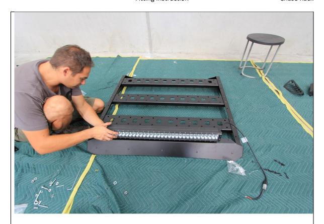
7. Light bars or other roof rack accessories can be fitted at this stage if required.
