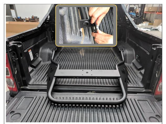
9. Lift tire carrier assembly into tub in preparation for fitment.
