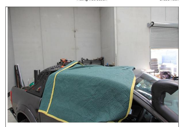
8. Prepare vehicle roof, by covering with a blanket or other soft protection sheet to prevent marking of roof.
