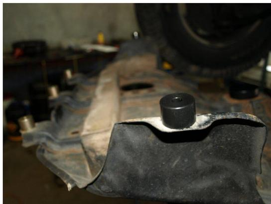
For these five locations use the supplied **M8xP1.25 x 40mm Bolts (H)** and **M8 Flat Washers (I)** – and on the front three spacers also use the **M8 Split Washers (J)**.
