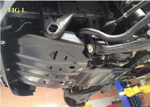
FIG1. Front factory bash plate to be removed—keep for refitting—modification will be required to refit..
