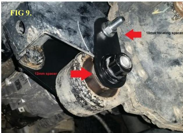
← FIG 9. Plate fitted to outside of bracket to locate diff mount, loosely install 10mm ID spacer and dome head M10x1.5px40mm bolt to original hole. Reuse the original 16mm bolt & nut with through bushing to bolt plate.
