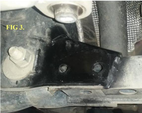
FIG 3. Once removed, clean the area with a flap disc and paint to avoid future corrosion.
