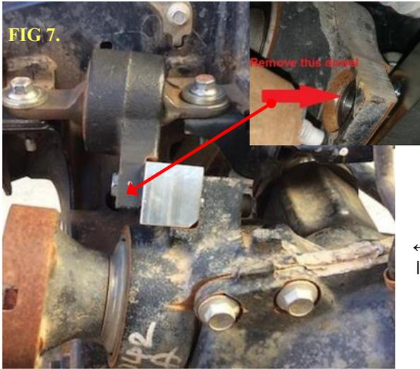
← FIG 7. Left hand rear upper most diff mount, unbolt forged diff mount from diff housing, and lower diff housing, remove dowel from diff mount (this must be removed to allow fitment), then install tapered block between diff mount and diff centre, applying a small amount of thread lock to the bolts supplied—M10 & M12 respectively (different size bolt per side of the block)
