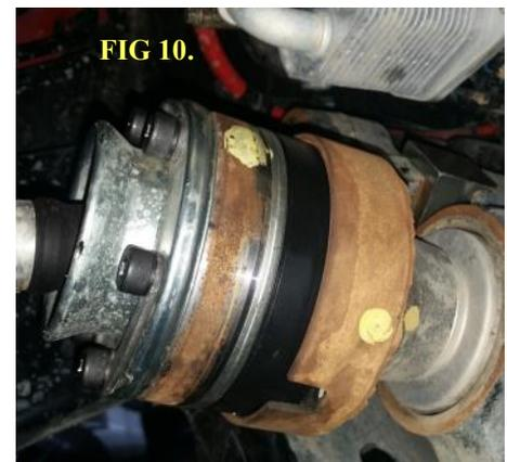
Once all components have been installed in the prescribed order, tighten all bolts to recommended torque values, re-install the bash plates. Now you have lowered the front diff mount, the bash plates will require spacing. Spacers for Bash Plate relocation are not included in the kit.—spacer requirements are specific to Bash Plate brand and design.
