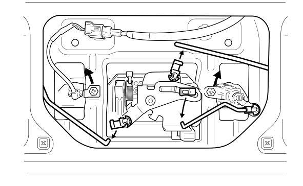
Fit Tail Lock bracket and indicated bolts. Then reconnect the previously removed rods.
