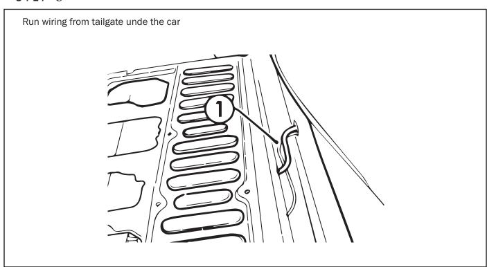
Run wiring from tailgate to front drivers side kick panel. Cable tie wiring every 500mm over chassis rail. Find the large grommet on the firewall, make a small incision & run the loom through it to enter the cab and towards the kick panel. Seal accordingly.
