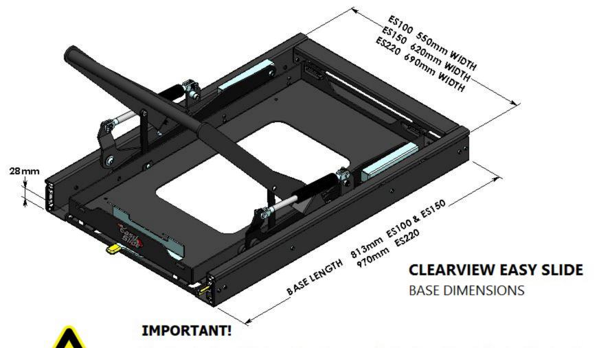
The Clearview Easy Slide base dimensions are critical in determining whether the Clearview Easy Slide will fit into your allocated space.
