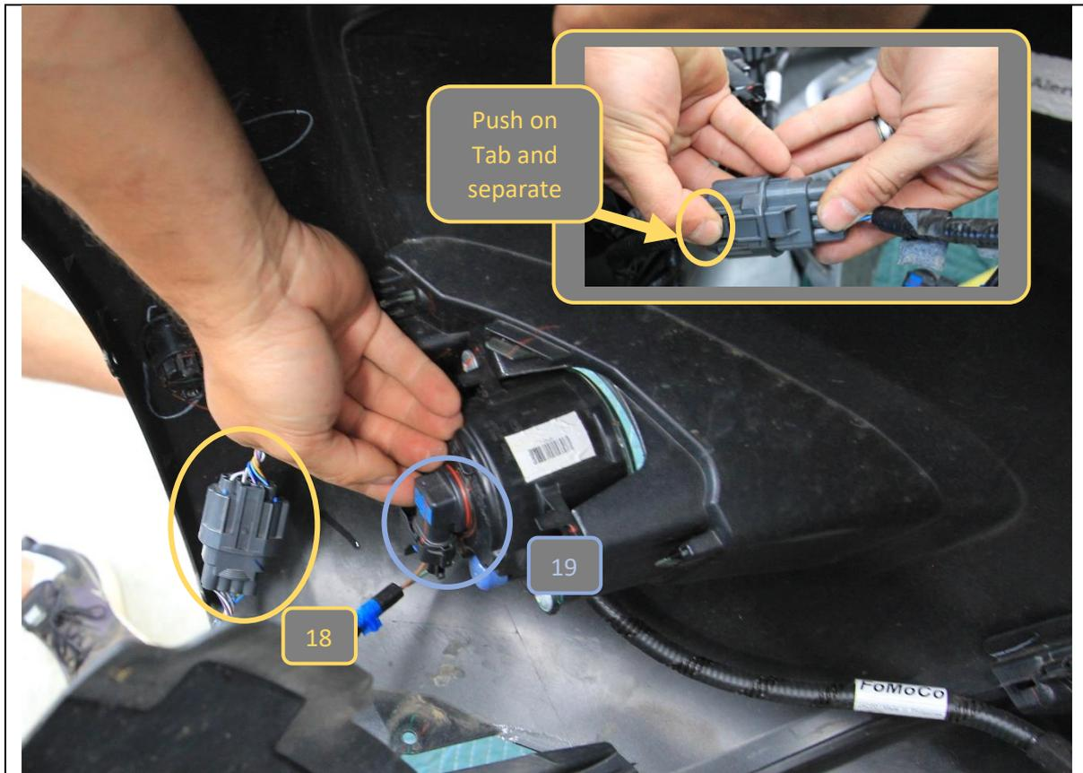
20. Disconnect the main parking sensor loom, on the front passenger side by pushing down on the tab and pulling the connector apart.
