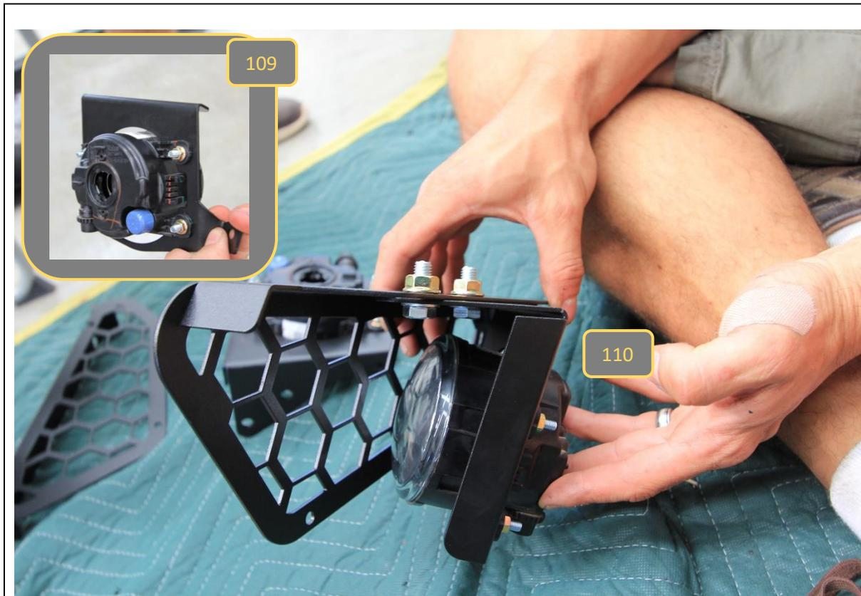
109. If re-fitting factory fog lamps, fit the fog lamps to the supplied fog lamp brackets using the M5x15 screws and Flange nuts provided.
