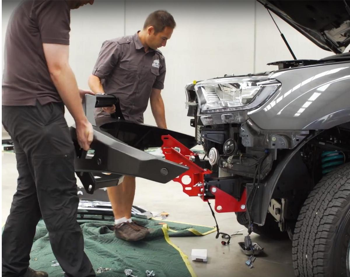
83. With assistance from either a lifting trolley or another person, Lift the bar up to the vehicle mounts.
