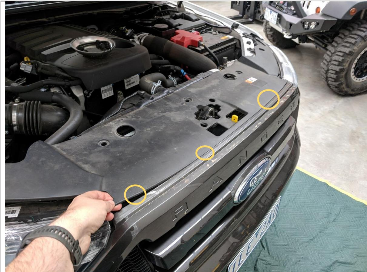
3. Carefully lift up plastic top shroud trim to unfasten concealed plastic clips securing trim to grille.
