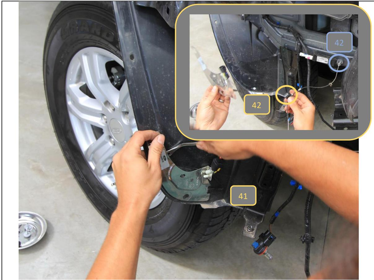
41. Remove the FM radio antenna from the lower section of the wheel arch liner on the driver's side, using a trim tool to pry it up.
