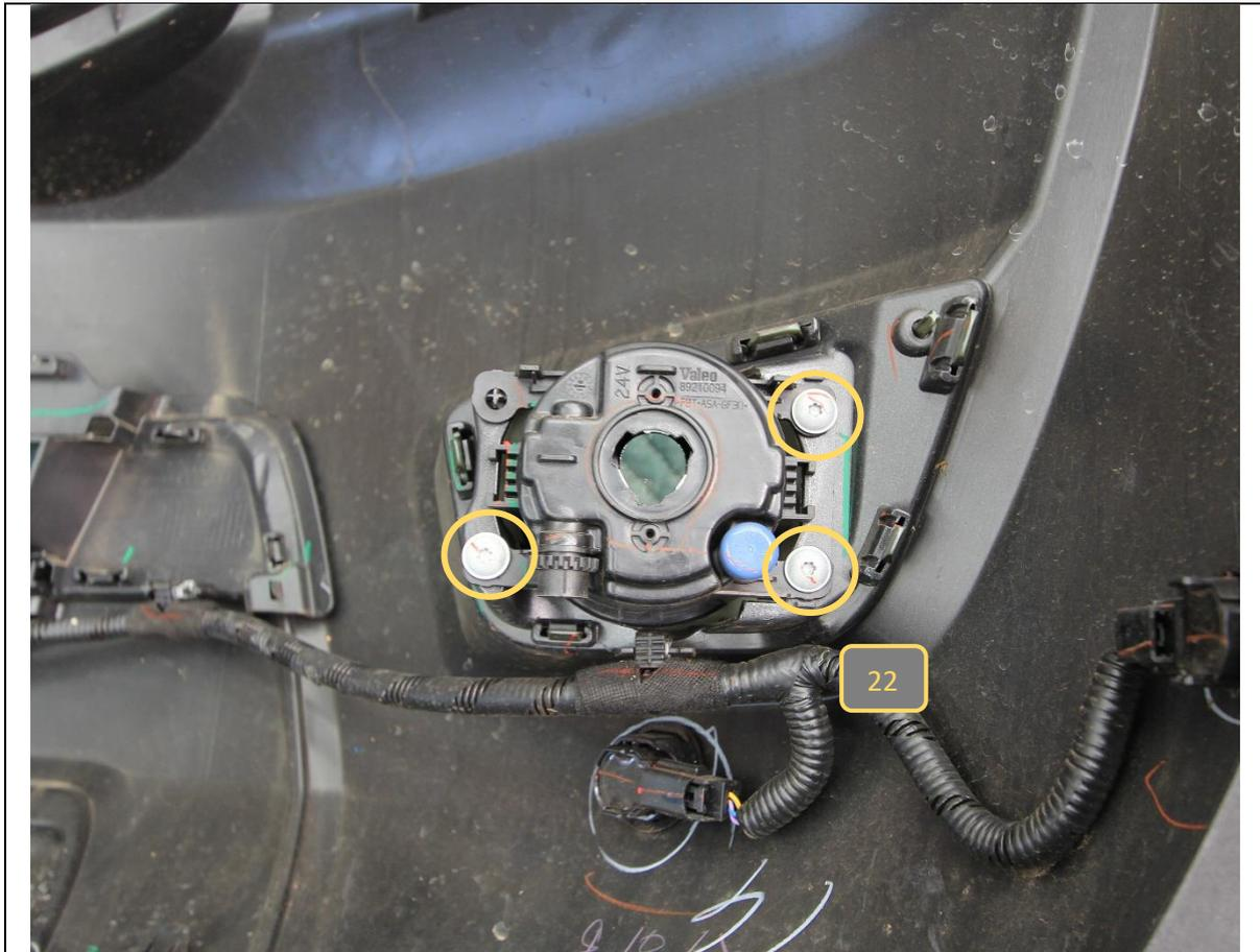
24. Remove fog lamp from bumper by removing the 3X T25 Torx screws.
