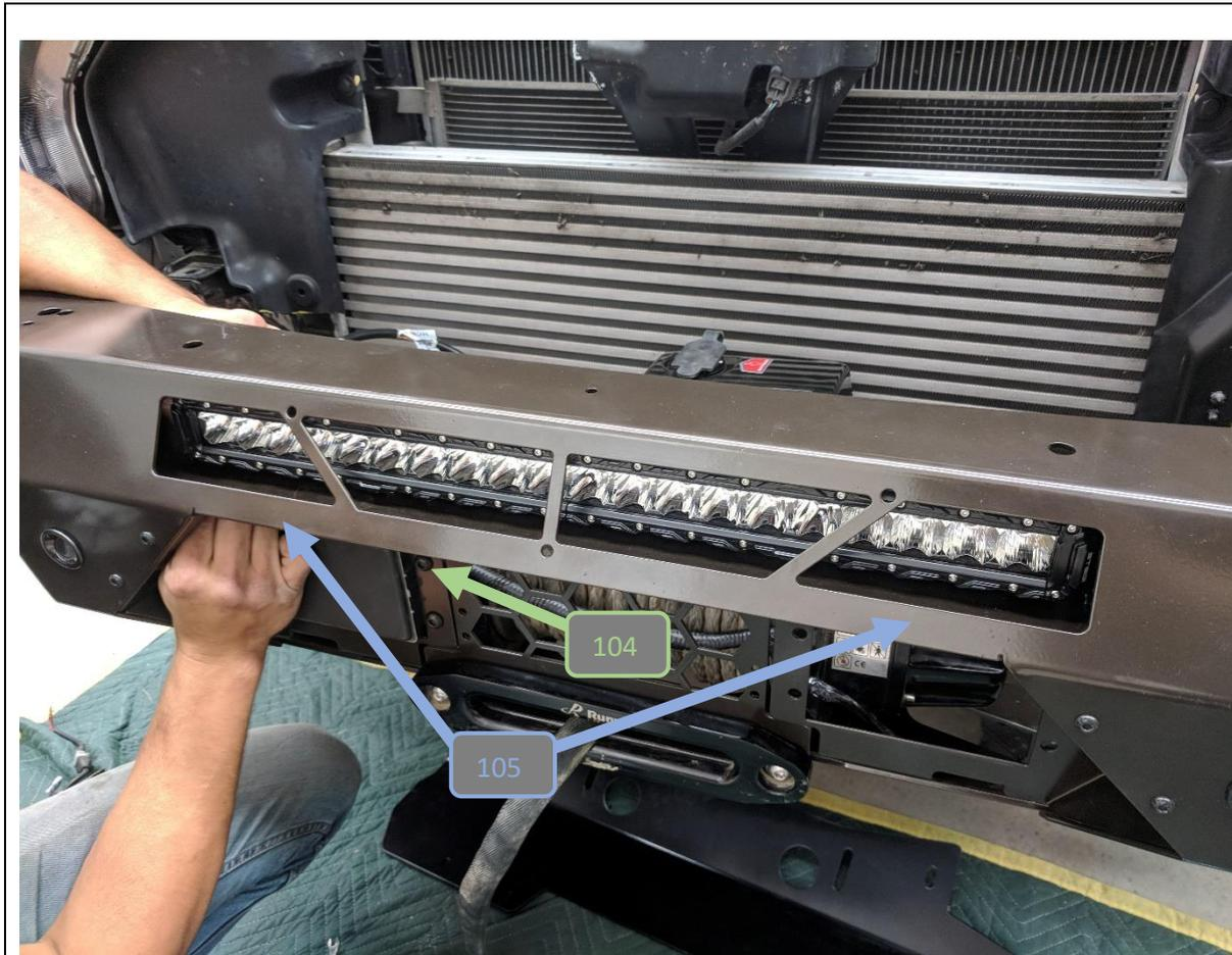
104. Reconnect wiring harness for adaptive cruise control sensor module
