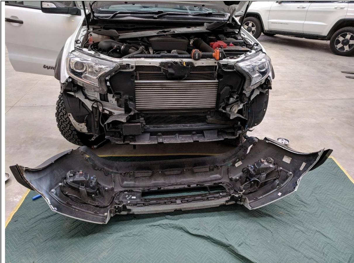
22. Once all clips are free and all wiring disconnected, lift the bumper off the car from the center section.
