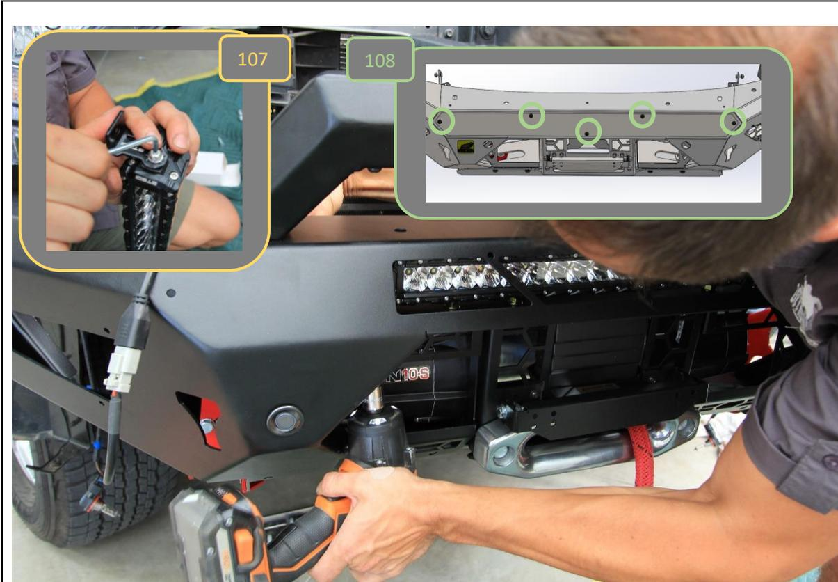
106. If fitting a light bar to the center section of the bar, do so at this stage.
