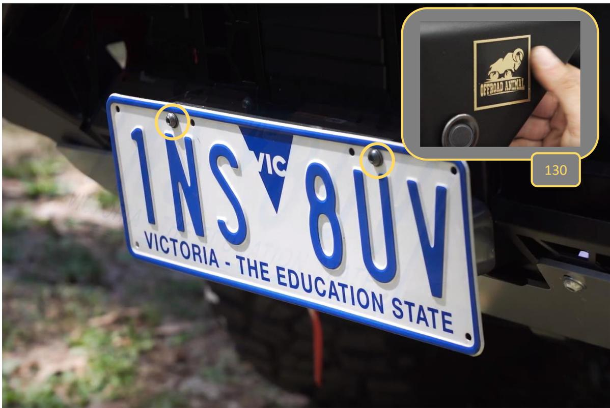
130. Re-Fit the number plate to the number plate flip, using the M5x15
