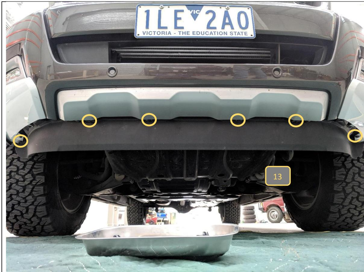
12. Remove the 6x Bolts securing lower bumper to the support brackets behind, using 8mm socket.
