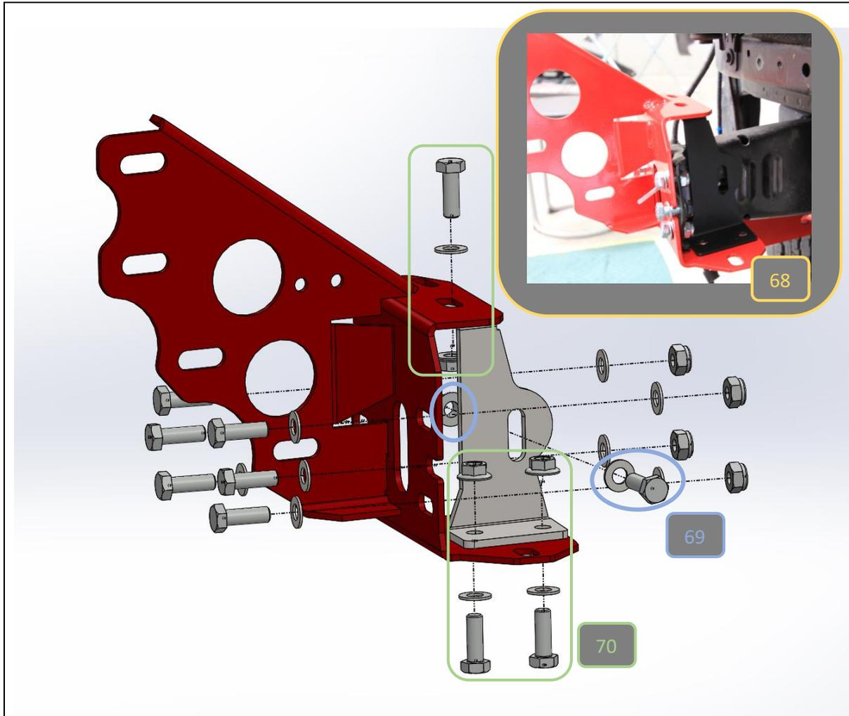
68. Fit Chassis bracket gusset to chassis and mounts.
