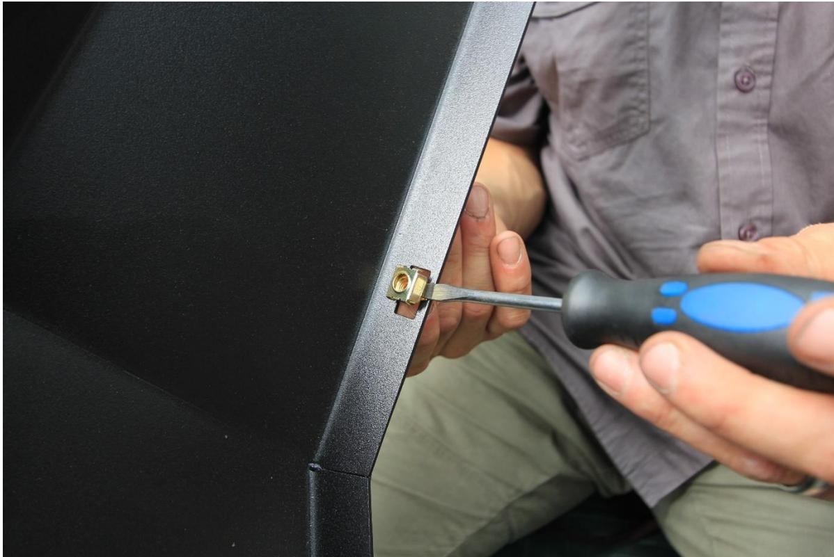
82. Insert cage nuts to square slots in bottom of wings. Seat cage nut against one edge of slot then push other edge in with flat bladed screwdriver.
