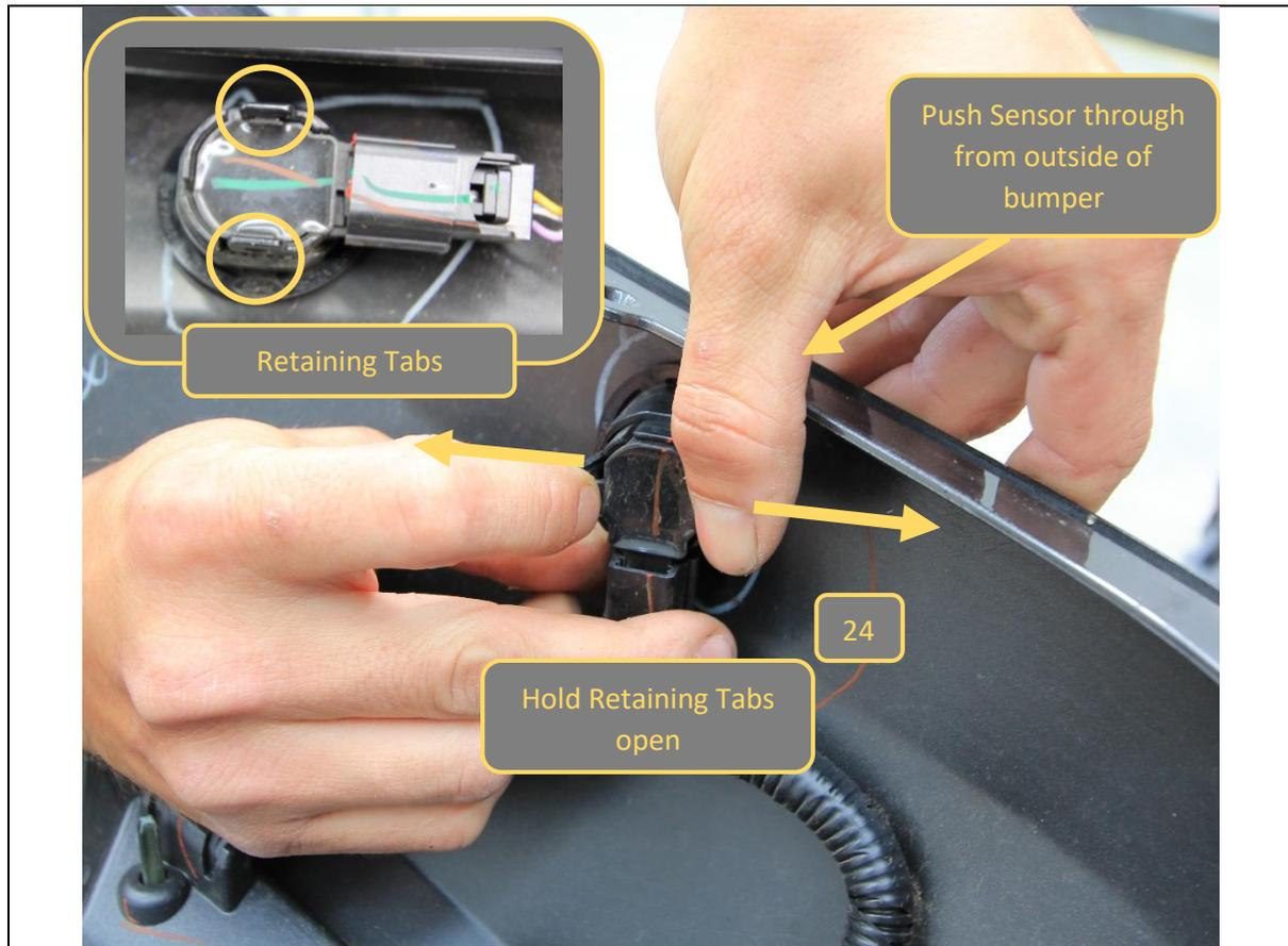
26. Remove parking sensors from housings, by holding open the retaining tabs, whilst pushing the sensor through the housing from the outside of the bumper
