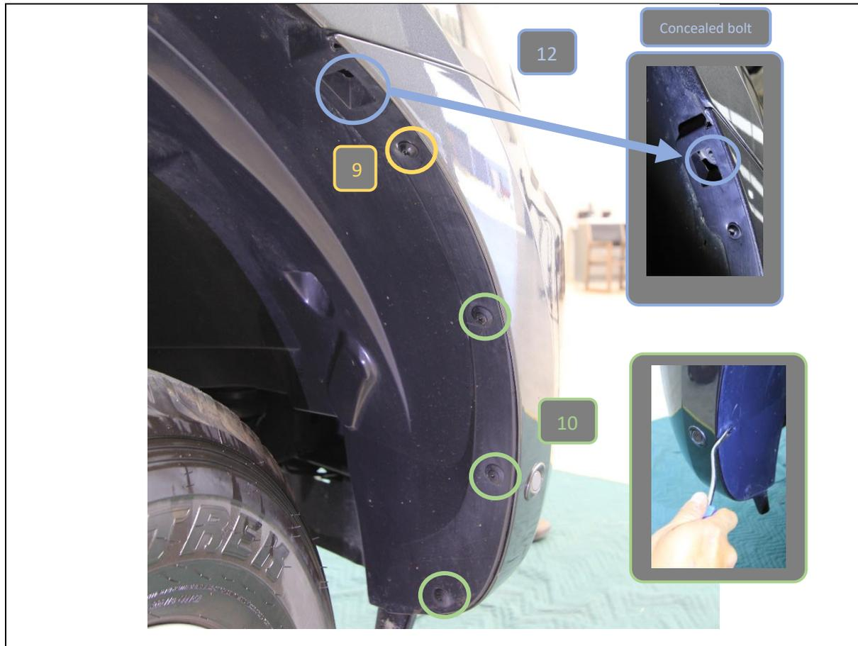
8. In the wheel arch remove the fasteners securing inner wheel arch liner to the bumper.
