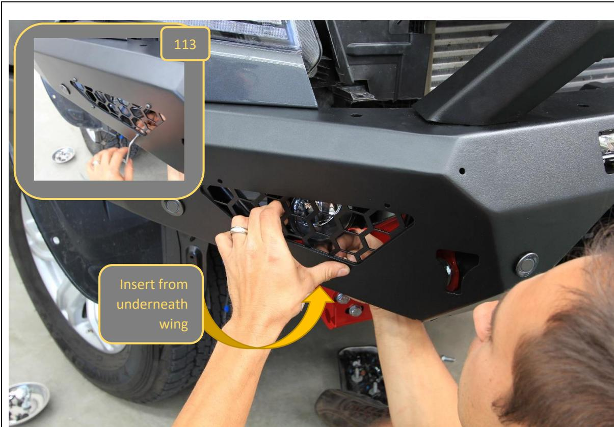
113. Fit light mesh panels to the bar. Position the panel from underneath the bar and align with the mounting holes in the wing. Secure with 4x M6x16mm Button head bolts and M6 Flange Nuts
