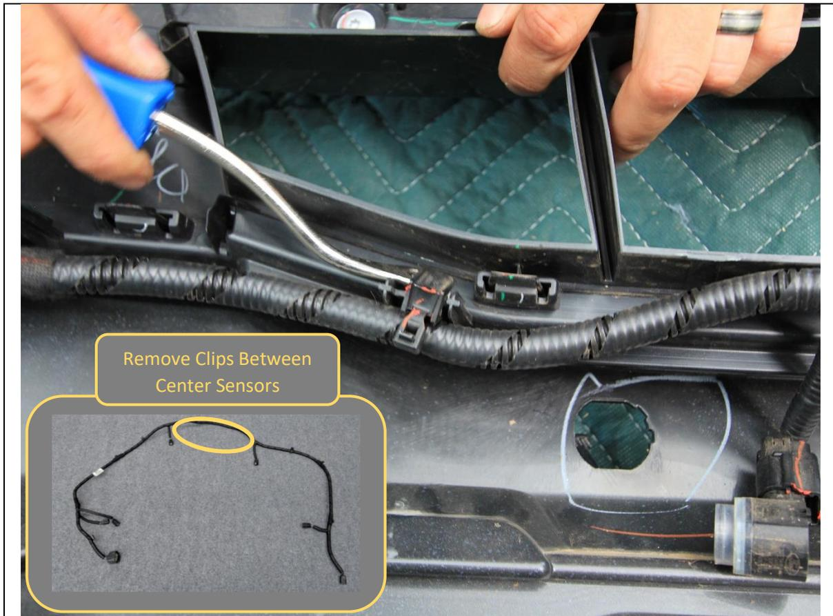
30. Separate parking sensor loom from bumper by prying off all the retaining clips using trim tool.
