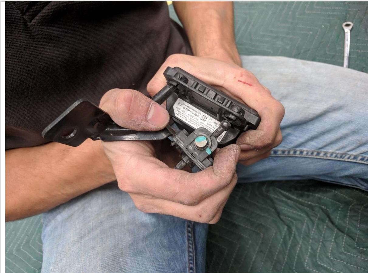
37. Separate the adaptive cruise control bracket from the support bracket by pulling the bracket out of the ball and socket clips.
