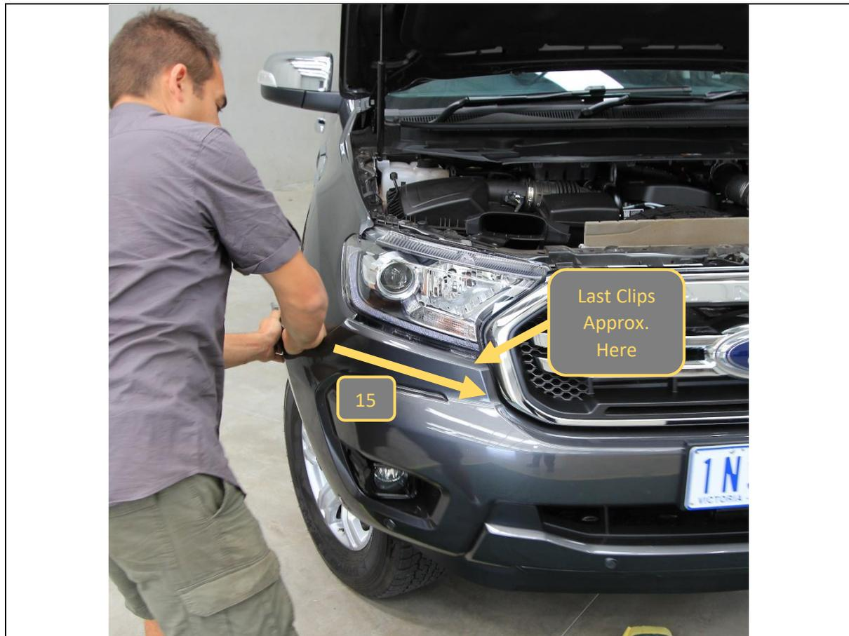
17. Starting at the wheel arch firmly but carefully pull the bumper away from the panel to release the clips.
