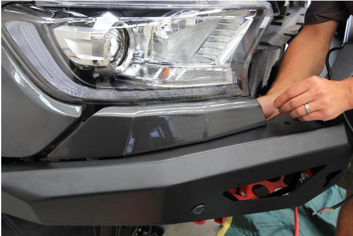
91. Fit headlight infill panels to the top of the wing, using M6x16 button head bolts, M6 flat washers and Flange nuts. Secure finger tight only at first.
