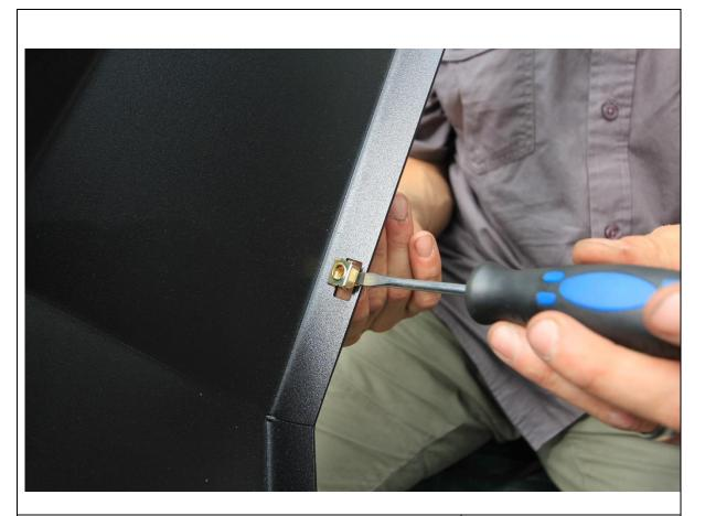
82. Insert cage nuts to square slots in bottom of wings. Seat cage nut against one edge of slot then push other edge in with flat bladed screwdriver.
