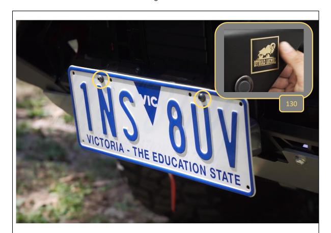
130. Re-Fit the number plate to the number plate flip, using the M5x15
