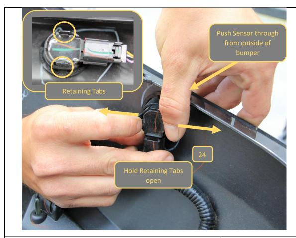
26. Remove parking sensors from housings, by holding open the retaining tabs, whilst pushing the sensor through the housing from the outside of the bumper
