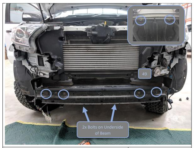
49. Remove the impact beam by removing the 4x M10 bolts securing it to the chassis and 2x bolts securing to bash plate, using a 15mm Socket.
