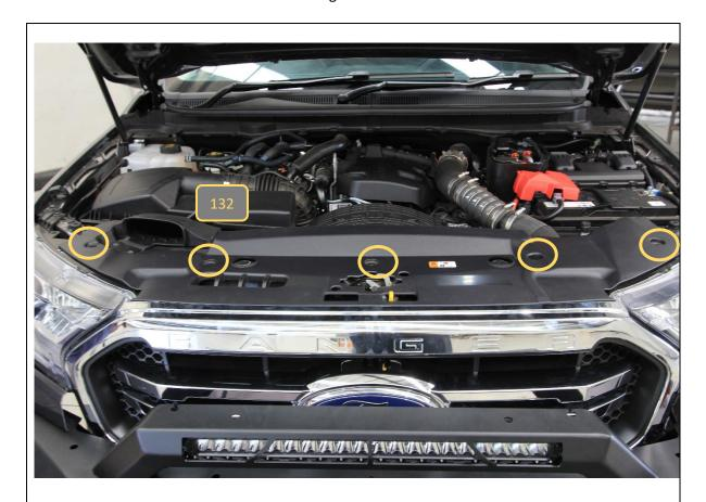
132. Replace plastic radiator trim. Replace 5x plastic push rivets inserting in hole, then pushing down center part.
