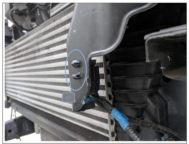
56. Re-Fit top portion of air guide using original bolt.
