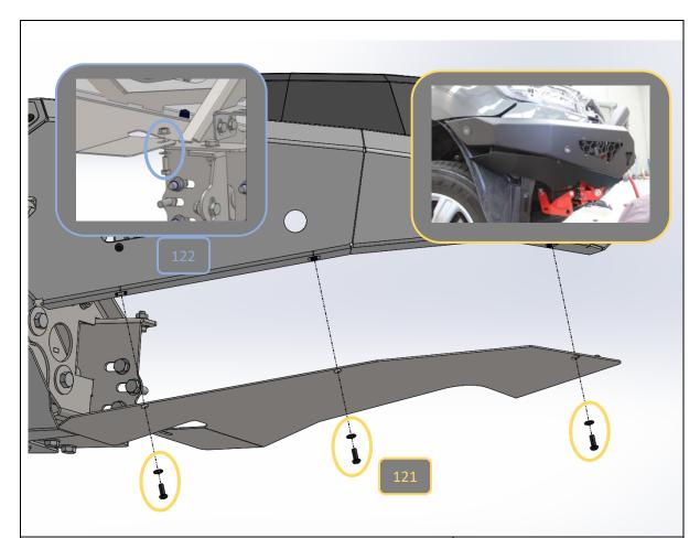
122. Fit side under panels to bar and secure with 3x M6x16 Button head bolts and M6 Flat washers, into M6 cage nuts fitted earlier.
