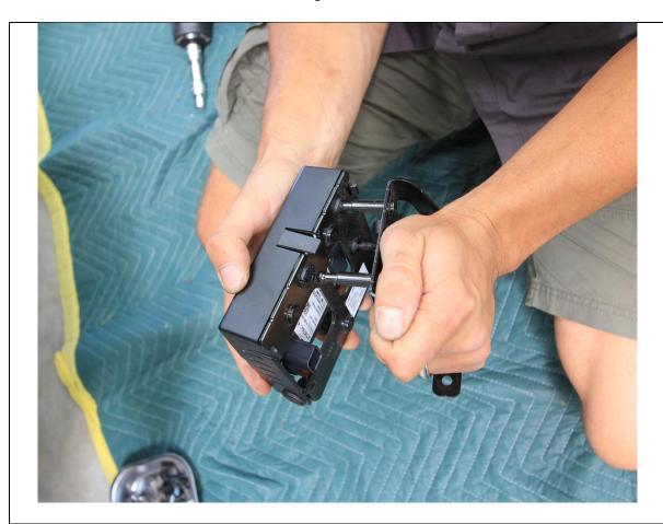
36. Separate the adaptive cruise control bracket from the support bracket by pulling the bracket out of the ball and socket clips.
