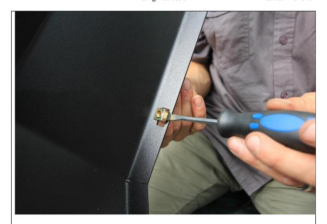
34. Using a flat head screw driver fit cage nuts to bottom edge of bar
