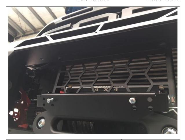
49. Fit centre mesh panel to bar with M8 x 16 black button head cap screw through the top and M8 x 20 black button head cap screws through bottom. Use washers and flange nuts
