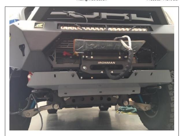
59. Fit front bash plate to lower section of bar. Insert part P-0072 shim plate between bar and bash plate. Use M8 x 30 button head cap screws, flat washers and flange nuts. Leave bolts loose TOOLS REQUIRED
