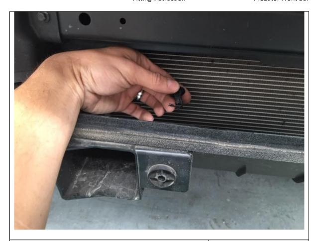
15. Remove plastic clips as shown, do this by pushing male section from outside to push clip back towards car (2 clips)
