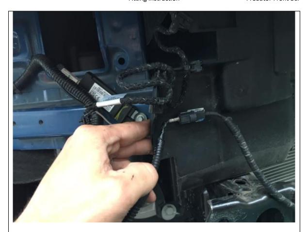
29. Push connector into new drilled holes as shown
