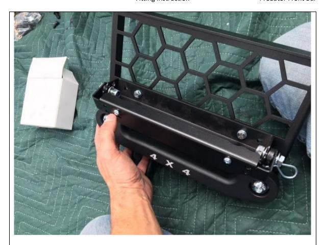
48. Fit Number plate flip bracket to centre panel with M6 hardware
