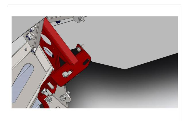
69. Secure inside edge of under panel to mount with M8 hardware
