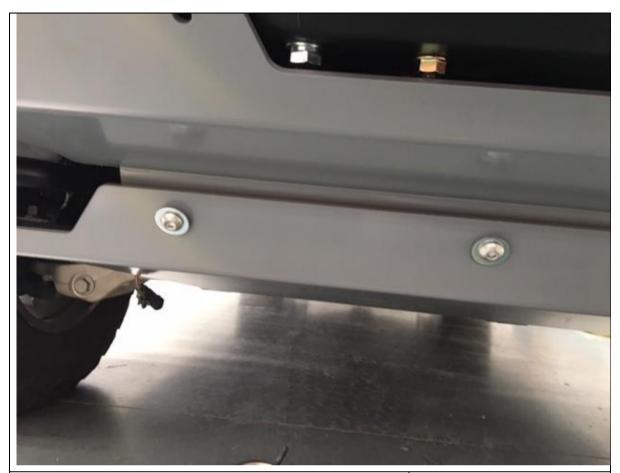
61. M10 button head cap screws tying in both bash plates shown
