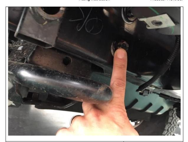
11. Remove 2 x M8 bolts per side as shown
