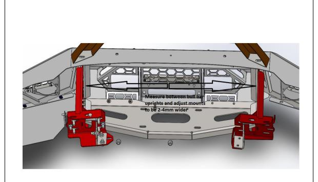
35. Measure bull bar between uprights and then adjust mounts to be 2mm-4mm wider.
