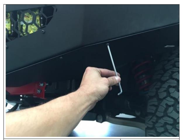
68. Position under panel on to bottom of wing and secure with M6 button head cap screws and washers
