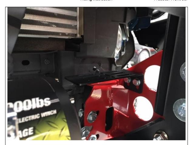
44. Depending on control box, ideal location is to mount on top of the winch, however if required fit winch control box mount as shown with
