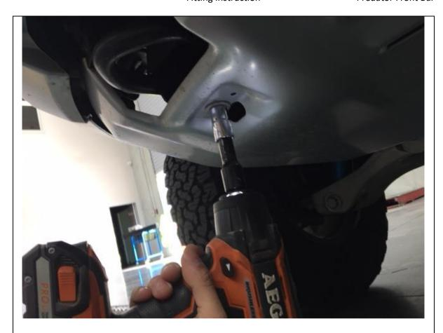
4. Remove factory bash plate (4 screws, 2 fwd and 2 at back)
