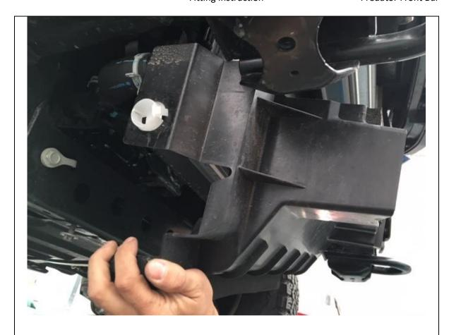
24. Time to remove lower air damn. See the white clip in the pic above, you need to pry this out from the inside of the chassis. One per side
