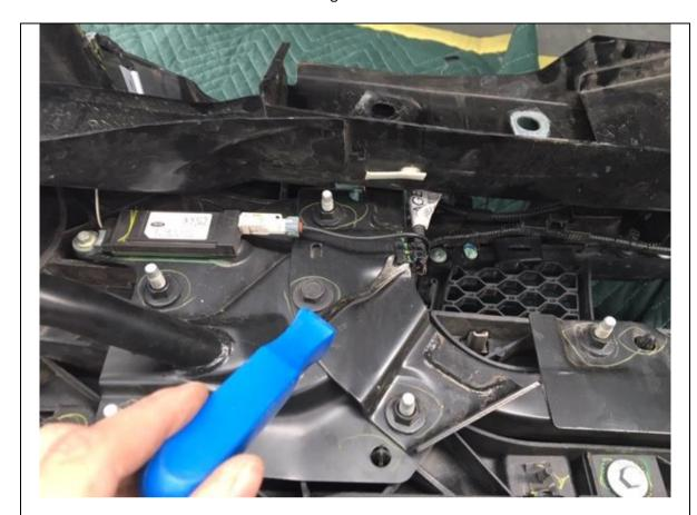
18. Pry out all cable/loom keeper for FM control box
