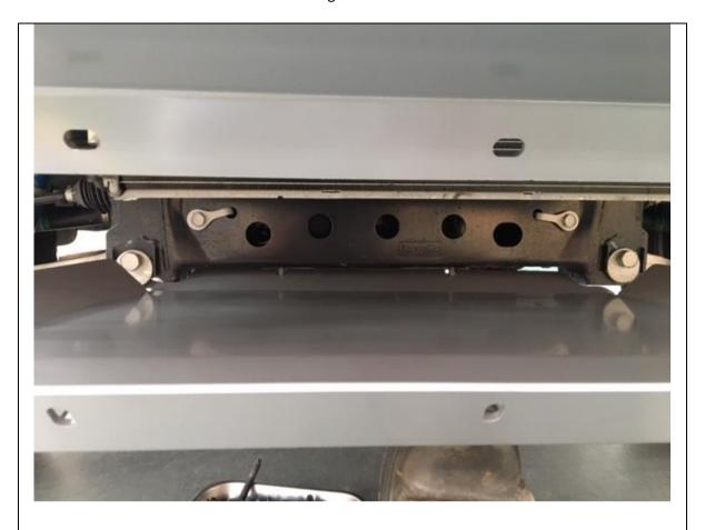
60. Time to fit new lower bash plate, with factory bolts started into threads at the back you can use them to hold up the back of the bash plate while you lift up the front and feed in M10 x 25 button head cap screws and washers.
