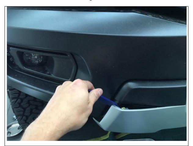
8. Using a trim tool pry off lower fascia as shown from both sides
