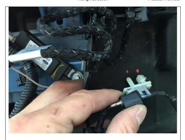
28. Relocate connector shown up on to plastic air damn guides as shown. Mark with paint pen then drill out with 6mm drill bit
