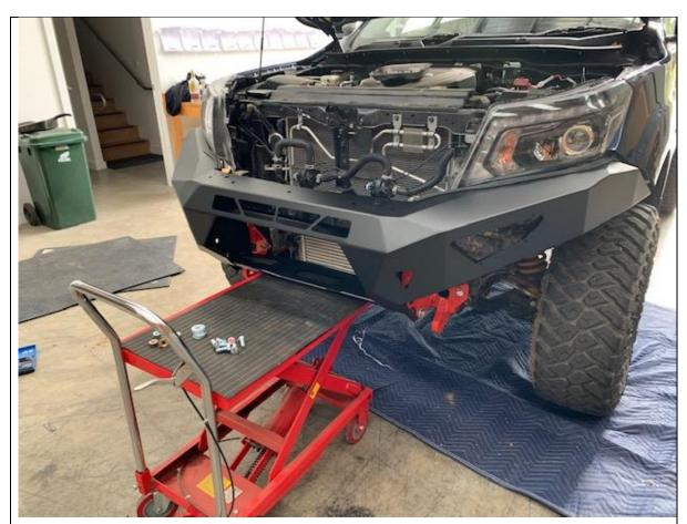
28. With the aid of a lifting table or a friend, lift bar onto vehicle
