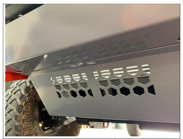
57. Fit secondary bash plate as shown. Use M10 hardware through both bash plates into mounts up top on sides. Reuse factory bolts on the bottom
