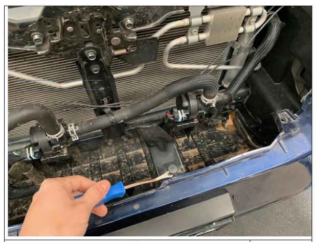
7. Remove all clips securing centre of bumper to vehicle
