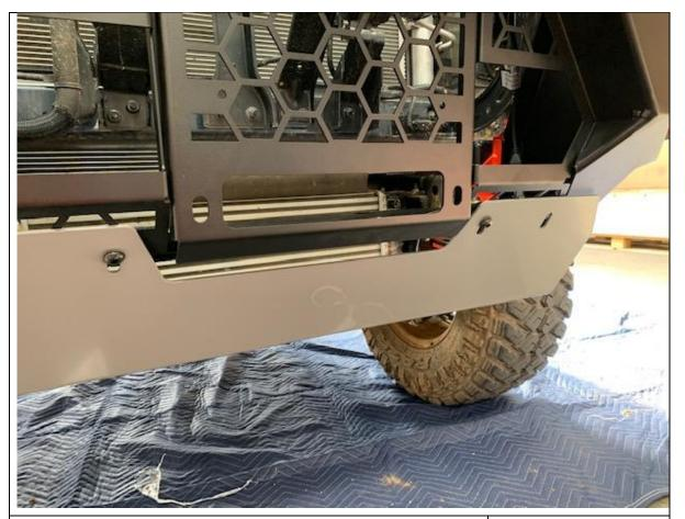
56. Fit Bash plate as shown with M8 x 30 BHCS washers and flange nuts. Leave off bottom bolts
