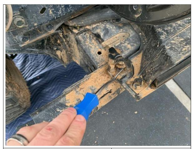
13. Remove lower air guide by removing 4 clips; 2 front (above) and 2 rear(below)
