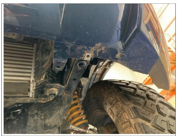
5. Remove factory bash plate and lower panels under bumper
