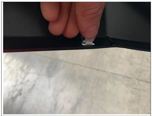
25. Fit cage nuts to bull bar by squeezing them in from above or using a flat head screwdriver to push them in
