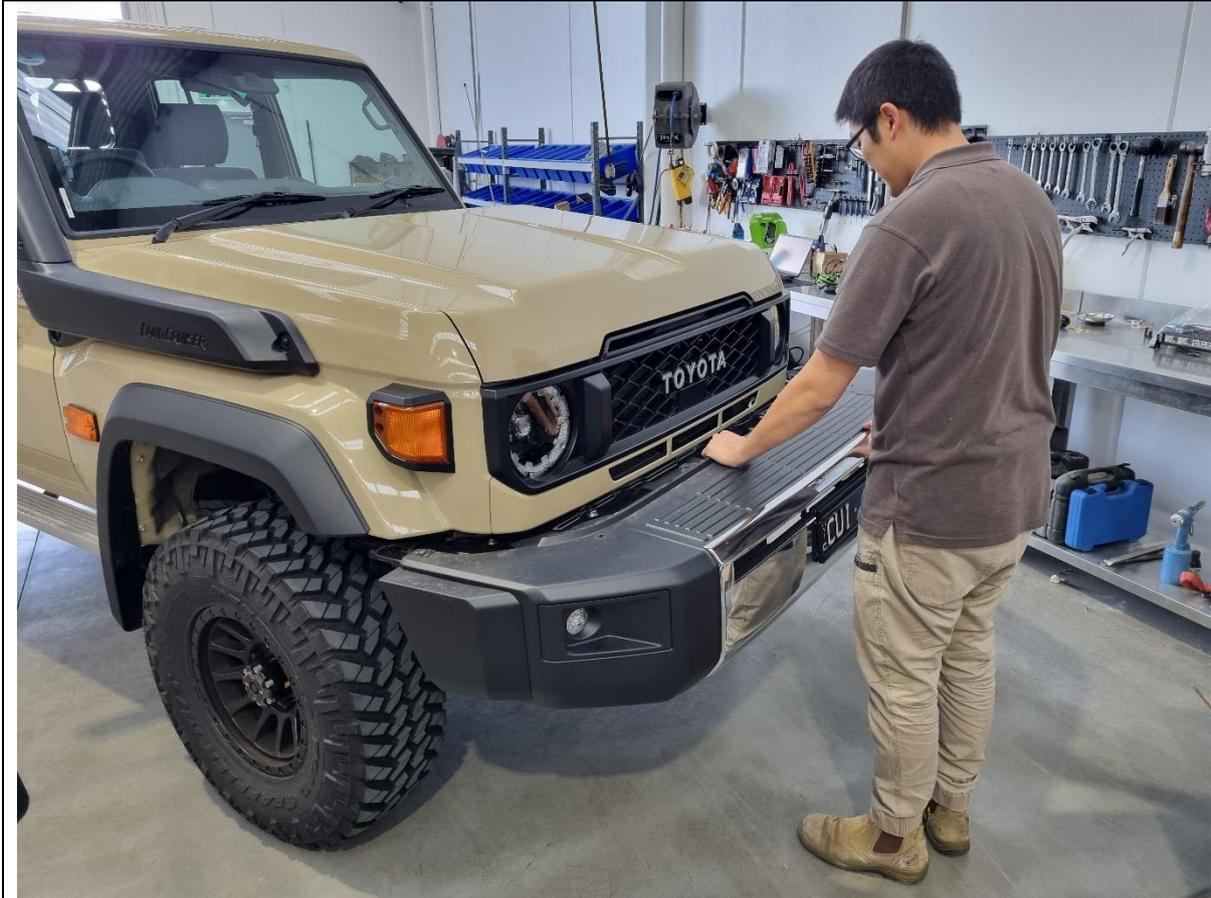
7. The bumper is now fully loose. Pull outwards and remove from vehicle.
