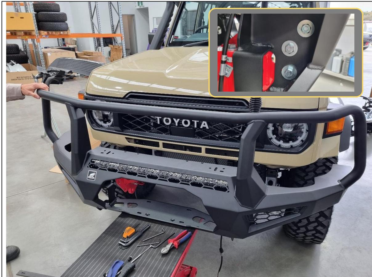
49. With assistance, either from another person, or a lifting trolley, lift the bar onto the mounts on the vehicle.
