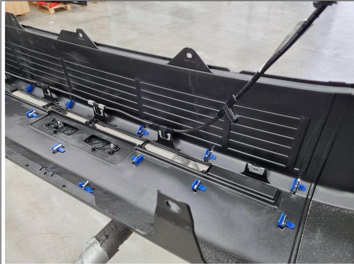
37. Unclip the loom from the bumper.
