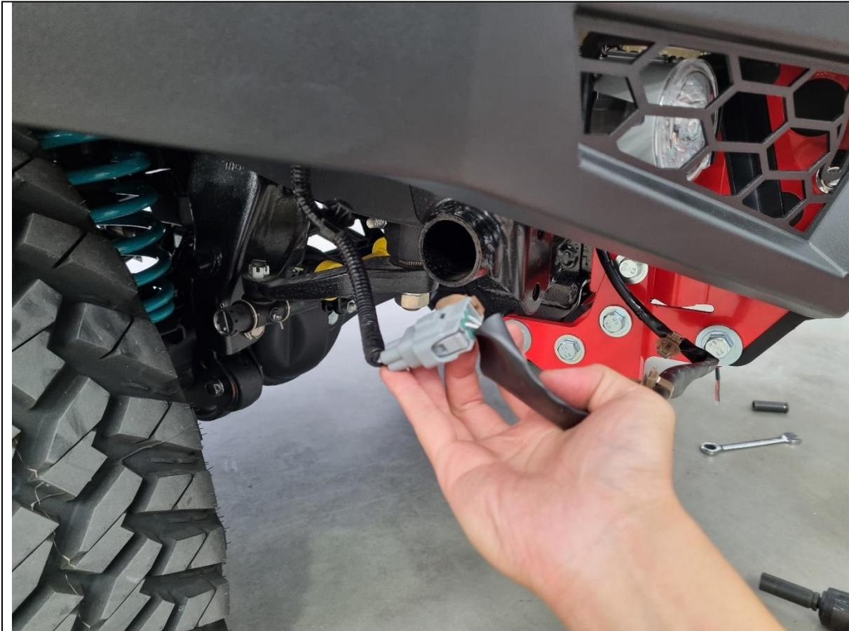
54. Reconnect the fog light and bumper loom to the vehicle.
