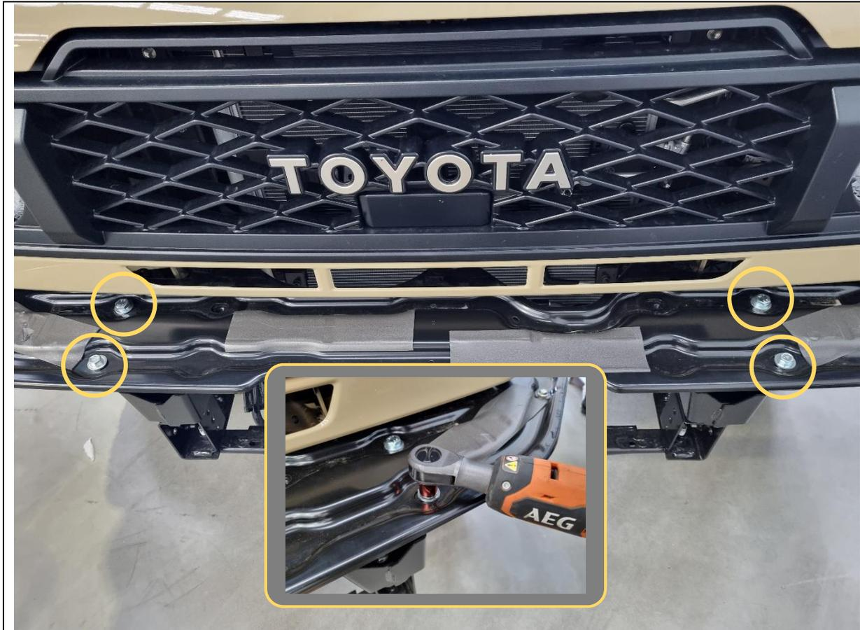
8. Remove the 4x 14mm hex bolts on the metal top panel.
