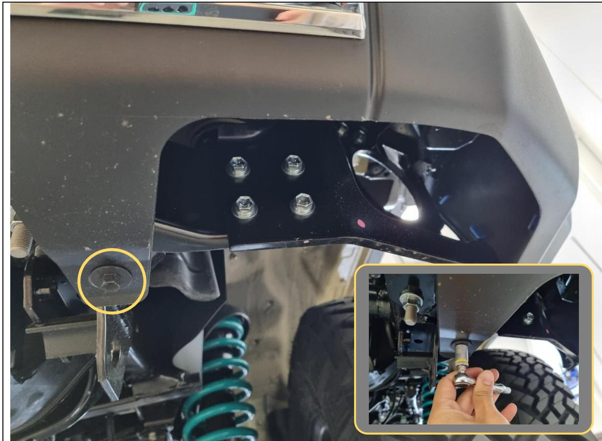
4. Remove 4x 10mm hex bolts along the underside of the plastic bumper.
