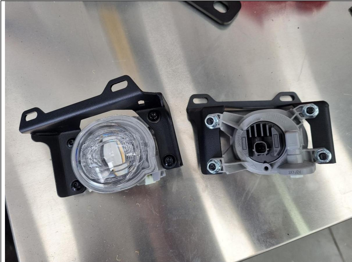
38. Fit the pair of fog lights to the supplied fog light brackets as shown.
