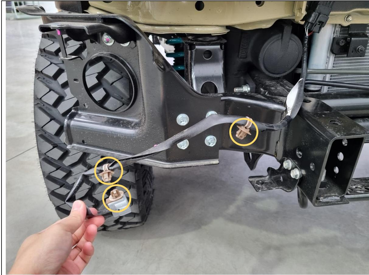
14. Unclip the bumper harness from the main impact bar.
