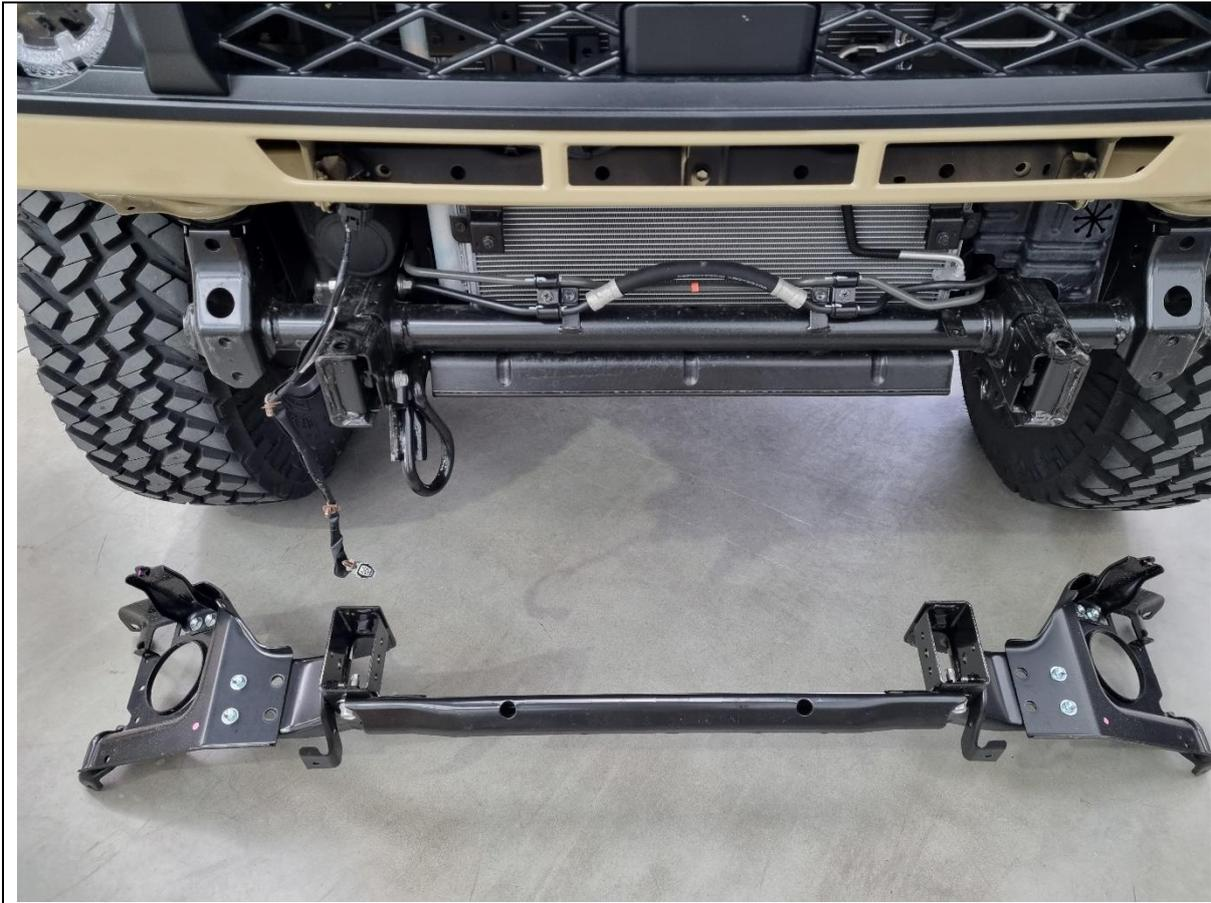
17. Remove the main impact bar from the vehicle.
