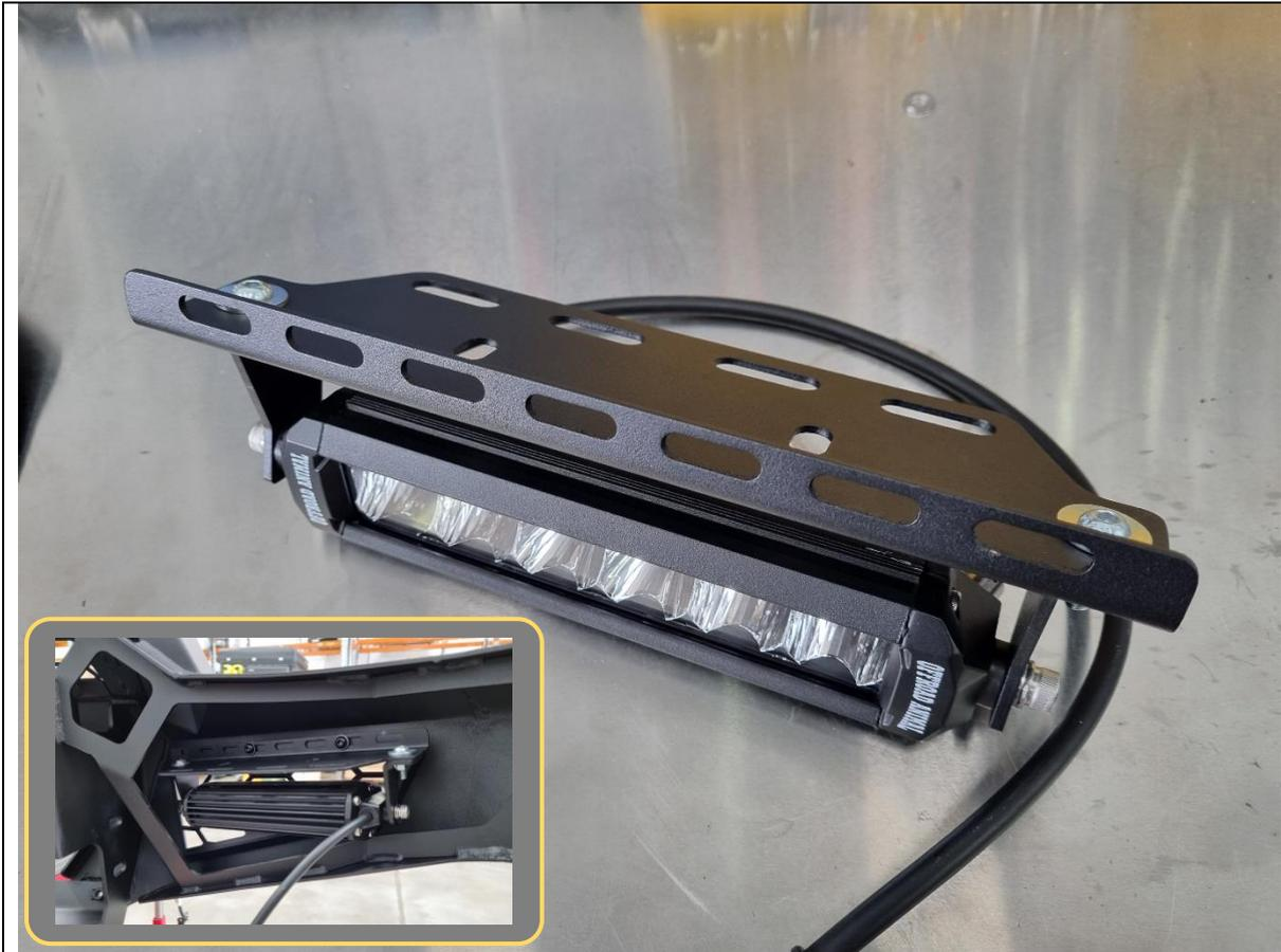
43. If not fitting factory fog lights, there is the option to fit Offroad Animal Halo Fog Lights (part no. ORA-ALO-M-2) with B-1185 mounting brackets (purchased separately), or fit 8" light bars or cube lights using the supplied B-1169 universal wing mesh light brackets (shown).
