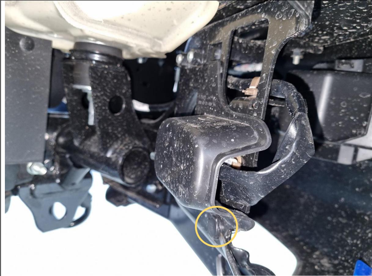
5. On the inside RH driver side wheel well, remove 1x plastic push clip holding the plastic cover for the bumper harness plug.
