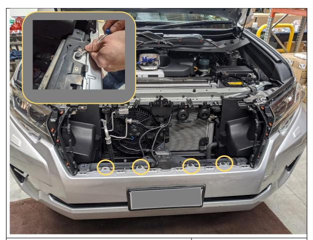
11. Remove the 4x Clips securing the bumper to the body crossmember
