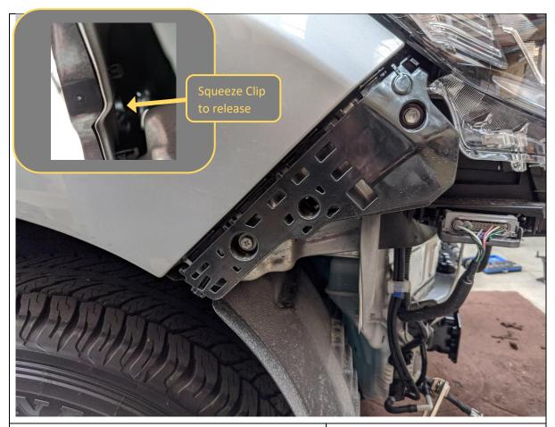
41. Remove the plastic bumper retainers by removing the Philips head and 10mm head screw, then prying out the large clip from behind using trim tool
