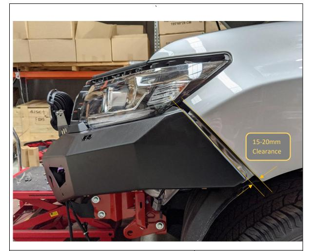
80. With assistance, from another person, Align the bar with the edges of the vehicle. Adjust such that the clearances are neat and even side to side.
