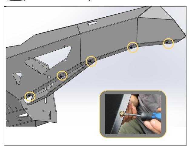
60. Fit 5x Cage nuts from small parts kit to rectangular slots in bottom of wing.
