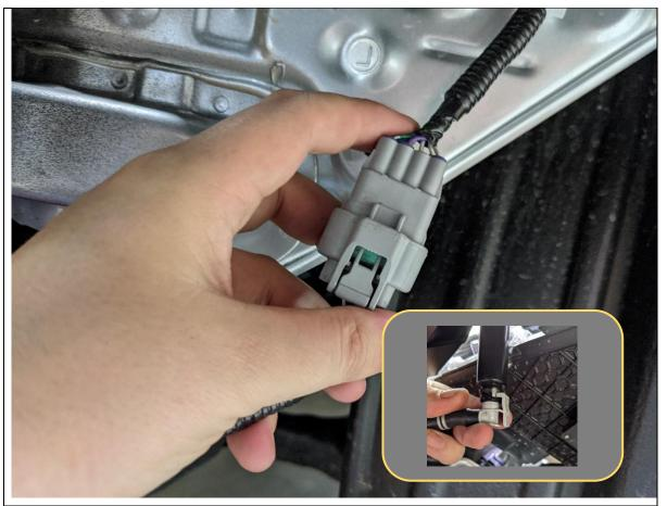
99. Re Connect Electrical Harness, fog lights and headlight washers. Make Sure to also reconnect Radar and Camera harnesses.
