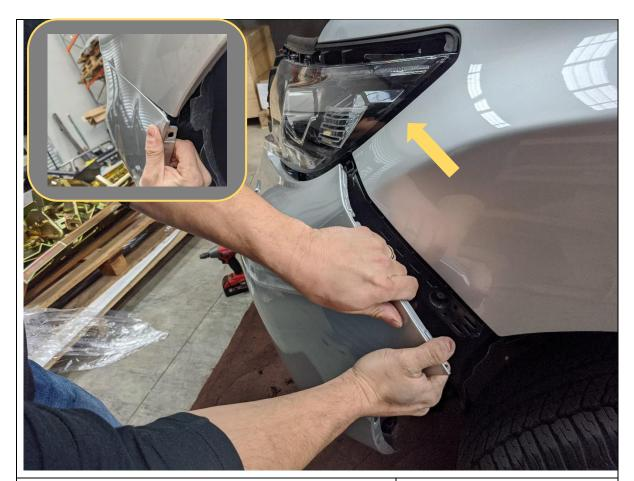
16. Starting from the wheel arch, carefully pull the bumper away from the body of the vehicle to release the clips.
