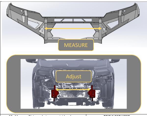
52. Measure Distance between outside edges uprights on bar using tape measure. Write distance below for reference if required.
