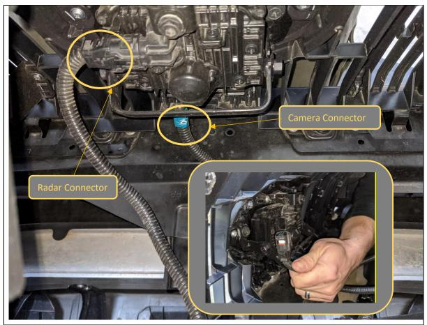
8. For Vehicles equipped with Adaptive cruise radar sensor and / or front camera, Disconnect the electrical harness connectors located on the back of the sensors.
