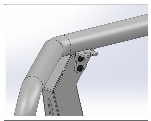
115. If fitting antenna to Torro bar, fit the antenna brackets to the M8 Threaded inserts in the uprights..
