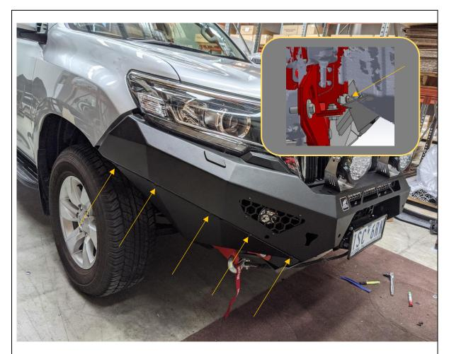
106. Fit Side Under panels (U-0029L/R) using, M6x16 button head and flat washer into the cage nuts placed earlier.
