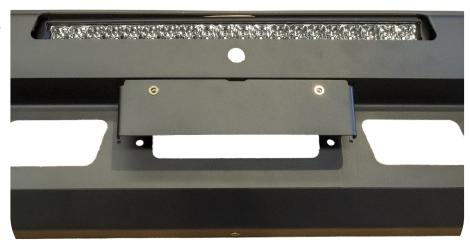
76. Place the nylon washer between the number plate bracket and the hawse mount. Tighten the nyloc nuts so that the number plate bracket can be moved using moderate force. DO NOT OVER TIGHT-EN.
