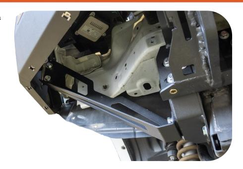
Secure the brace to the chassis support bracket using four M10 x 1.5 x 30mm hex bolts, M10 spring and flat washers.
