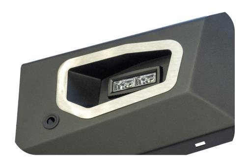
80. Secure the light trims to the outer sections with M6 flat washers and M6 nyloc nuts.
