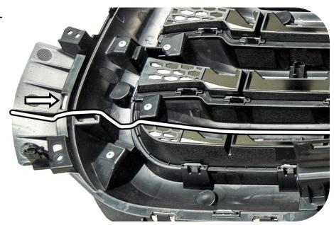
54. Using a multi-tool, carefully trim the grille along the line as described in the above steps.
