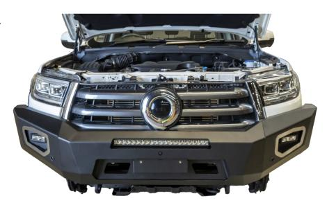
89. Secure the bar to the chassis mounts using six M12 x 35mm hex bolts, six M12 spring washers, twelve M12 flat washers, and six M12 hex nuts. Tighten enough so that the bar is secure but still able to be adjusted.
