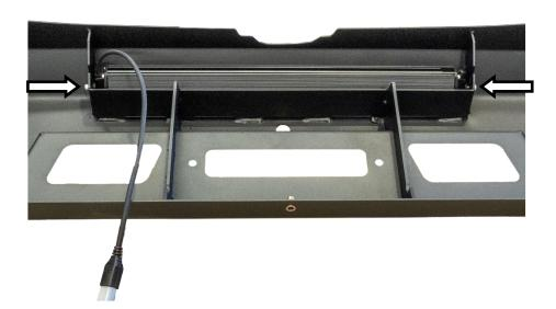
71. Fit the camera, or camera blank (removed earlier), to the camera relocation bracket (item 18) using two M5 pan head screws, four M5 flat washers and M5 nyloc nuts.
