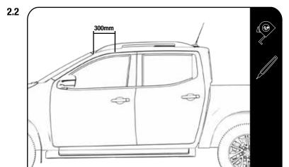
Starting at the top edge of the vehicle's windscreen, measure and mark the dimension as shown in 2.2 onto both LH / RH ditch centre's.
