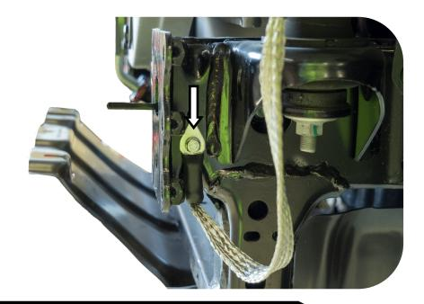
25. Remove the earth strap from the right hand chassis rail. Retain the fastener for re-fitment.
