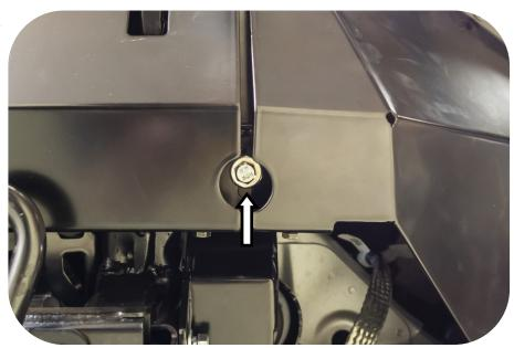
112. Fit the number plate to the bar or pivoting number plate bracket using two M6 pan head screws.
