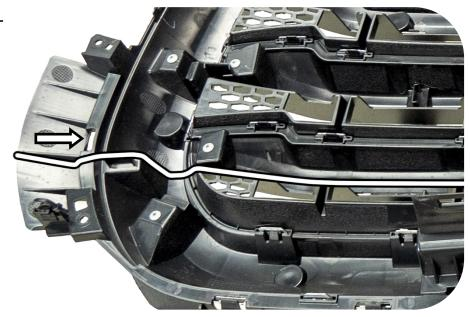
58. Using a multi-tool, carefully trim the grille along the line as described in the above steps.
