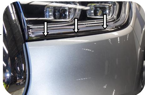
15. Remove the bumper bar and grille assembly from the vehicle.
