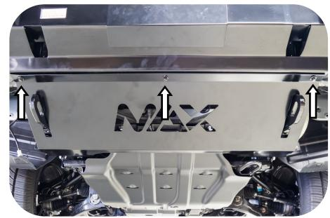
104. Secure the rear of the stone tray to the stone tray mount brackets with two M6 x 20mm hex bolts, M6 spring and panel washers.
