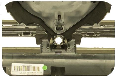
46. Remove the fog lights from the bumper bar to gain access to the front parking sensors.
