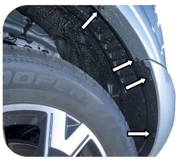
9. Remove and retain the fasteners securing the inner guards.
