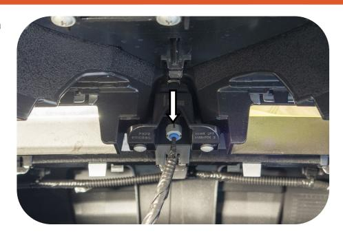
8. Remove the four fasteners (both sides) connecting the bumper to the inner guard. Retain the top fastener.
