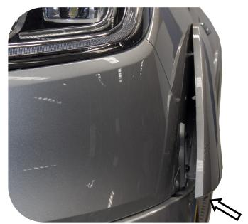
12. Behind the flares, remove and discard the two screws (each side) securing the bumper bar to the vehicle.
