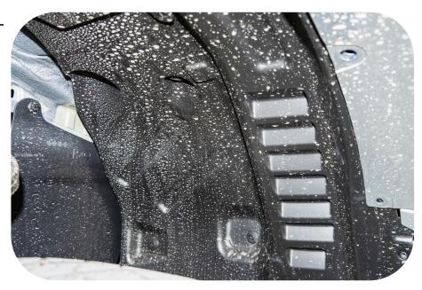
10. From underneath, remove and discard the fasteners retaining the bumper bar to the vehicle.
