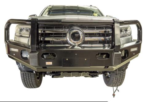
86. Secure the bar to the chassis mounts using six M12 x 35mm hex bolts, six M12 spring washers, twelve M12 flat washers, and six M12 hex nuts. Tighten enough so that the bar is secure but still able to be adjusted.
