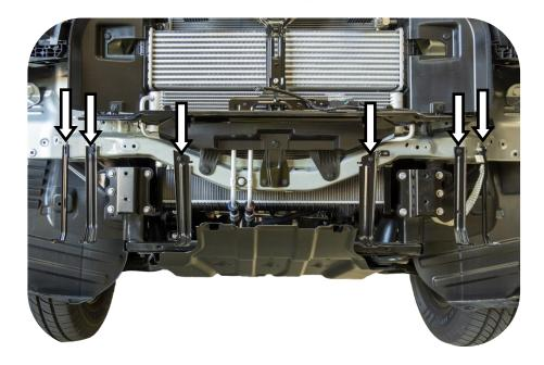
20. Remove and discard the two chassis end brackets. Retain the fasteners for fitment of the chassis mount.
