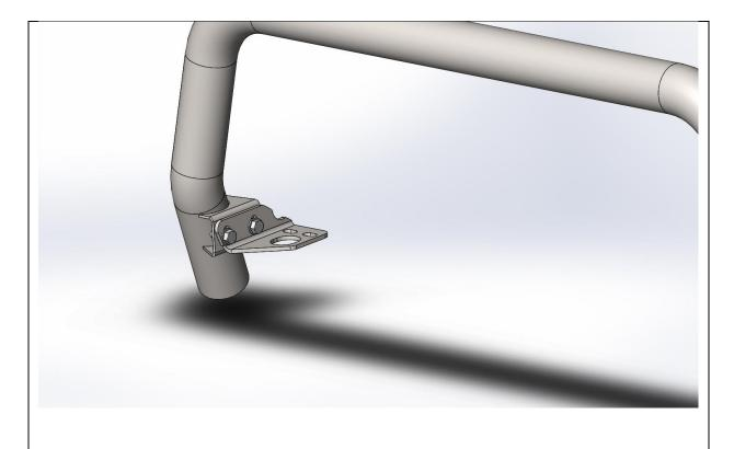
10. Loosely fit Mount brackets to nudge bar with M10 x 25 Hex bolts, washers and flange nuts
