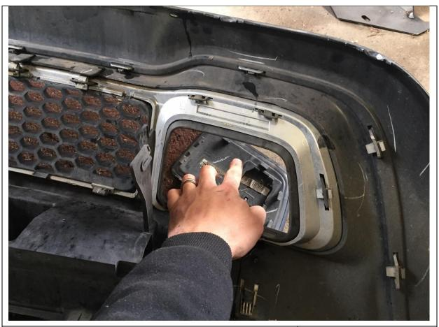
8. Push out panels to allow tow points to pass through. If yours do not push out, you will need to cut an access window in this area
