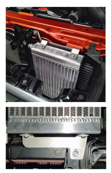
The horn bracket locating tabs will need to be bent flat, then fitted under the left mounting screw as shown. Once mounted, bend the horn bracket downwards to allow clearance for the grille, by gently pushing down on the horn. Ensure all screws are tight, & reconnect horn wiring.
