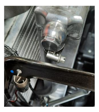
Once all components are installed and secure check for leaks and rattles by starting the vehicle and go over the whole installation process. It will be neccesary to either fill up the transmission with more oil due to the extra volume of the oil cooler unit, or depending on kms, perform a full transmission service. Follow the manufacturers specifications and procedures to ensure the process is performed correctly.
