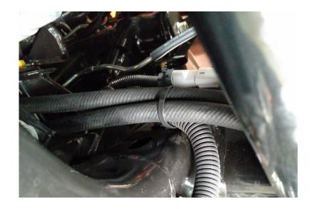
Fit the supplied P-Clip with M6 bolt, washers & nut, to the front of the chassis as indicated on image right. Keep hoses clear of the front swaybar.
