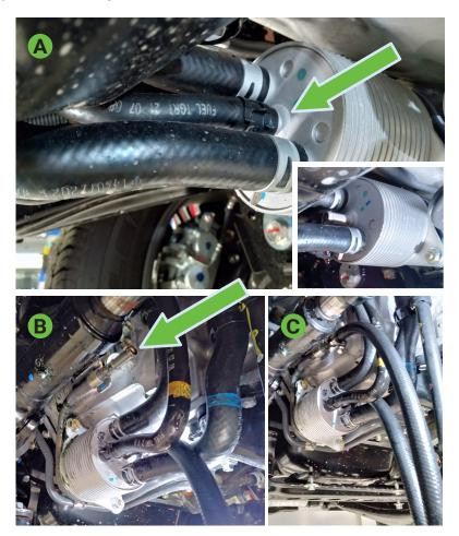
Route new hoses from the factory heat exchanger to the front of the vehicle where the new transmission cooler is located
