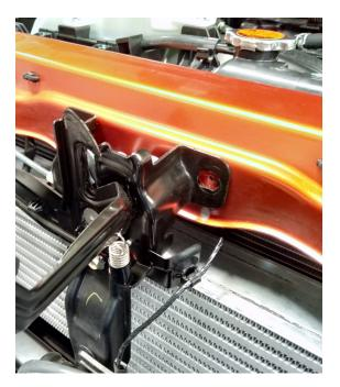
Fit the new supplied upper mounting bracket to the top of the radiator support where the bolt for the bonnet latch and horn were removed using the original bolts, as shown in the picture below.
