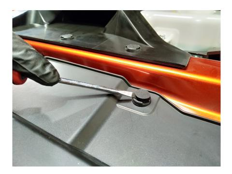
With the top cowling removed from the vehicle, there are some panel clips holding in the grille which need to be removed, as well as a central screw in the grille. The grille can now be lifted up & out of the way.
