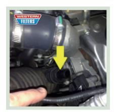
STEP 2: Run second hose with 90 degree hose end and connect to air intake fitting near turbo.
