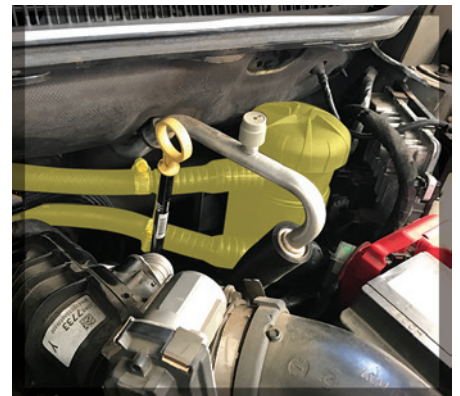
Image of Provent Kit Installed
