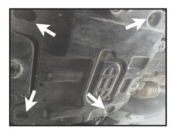
tip - make note of  $4\ x$  threads holding factory sump guard. These  $4\ x$  threads will be used to mount your Bushskinz Sump Guard in Section 2
