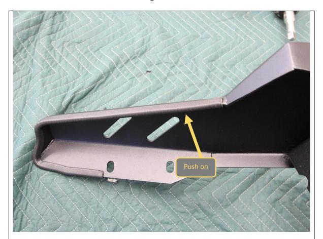
29. Fit rubber pinch weld to lower edges of wing, in the location shown by pushing rubber over the edge.
