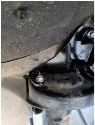
3. Reinstall the bump stop using the original bolts, bolting through the new bracket. Leave them slightly loose.
