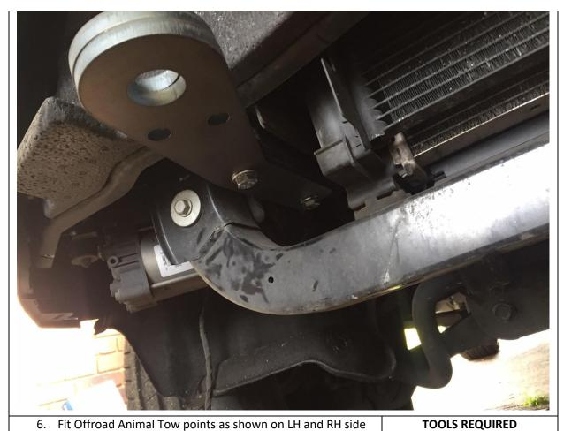
6. Fit Offroad Animal Tow points as shown on LH and RH side with M10x80 bolts directly into frame of Jeep. Torque down bolts
