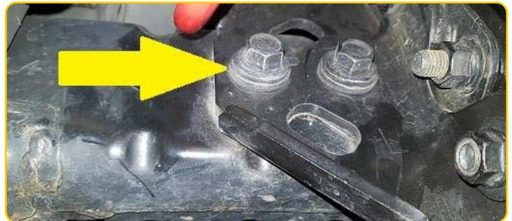
5. This small protruding tab needs to be bent in out of the way for the supplied crush sleeve to fit in.
