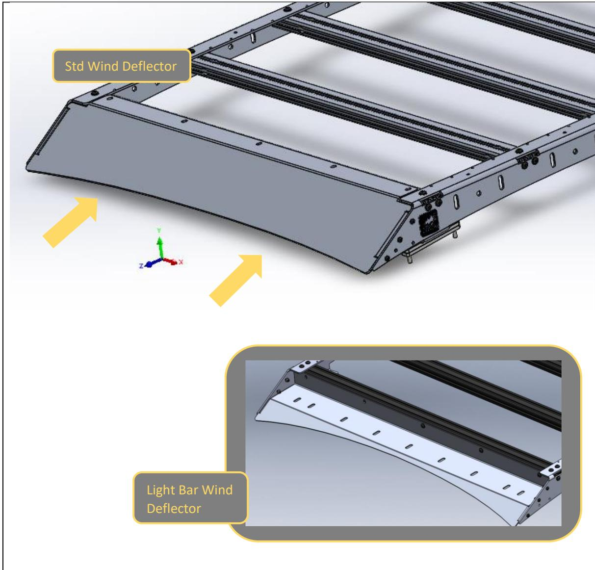
27. Fit the wind deflector to the rack assembly. The deflector should sit inside the side rails and on top of (Standard type) or in front (Light bar type) the first extrusion member.
