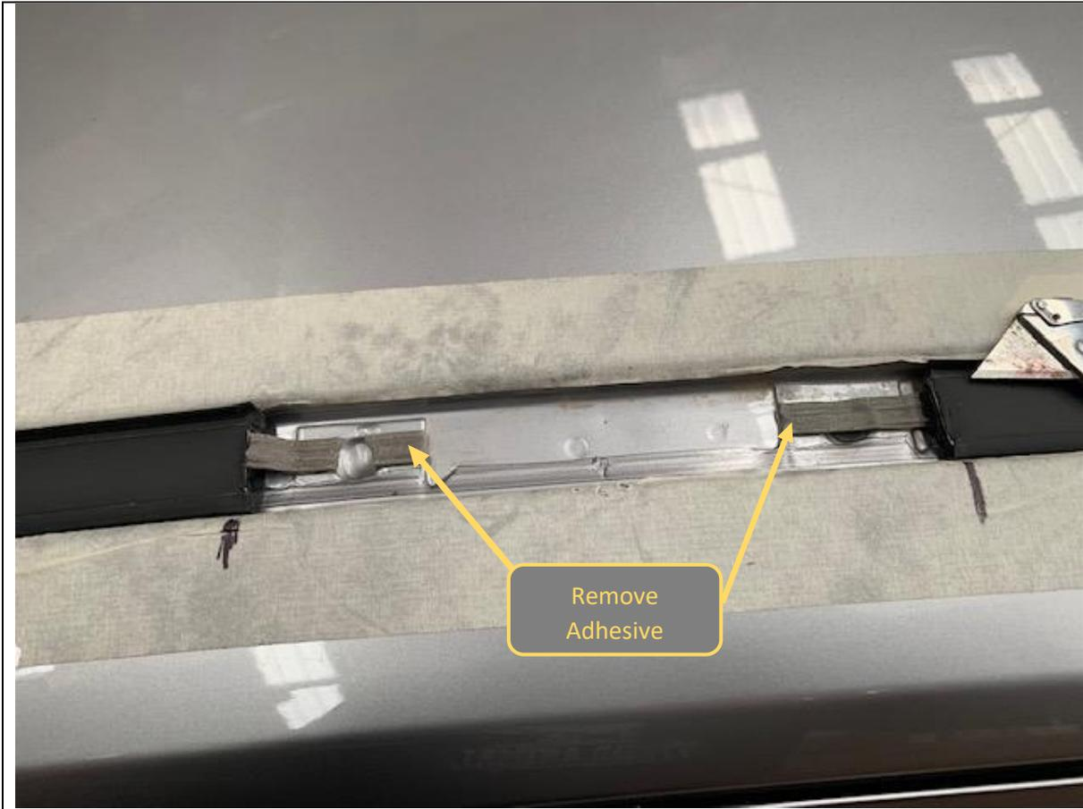
4. Carefully Remove the remaining adhesive tape, using a utility knife.
