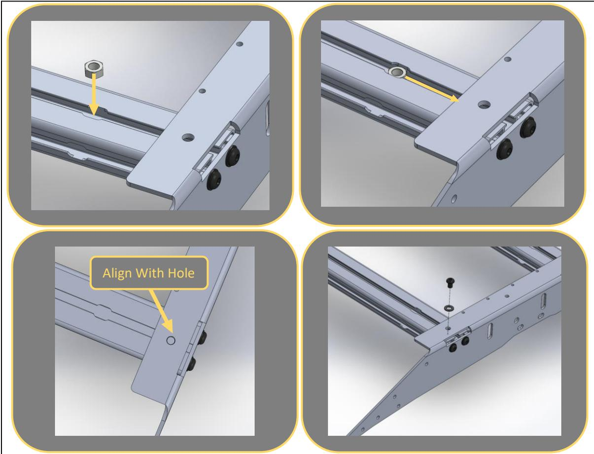
20. Insert M8 Nut into each track for securing top face of side rail.
