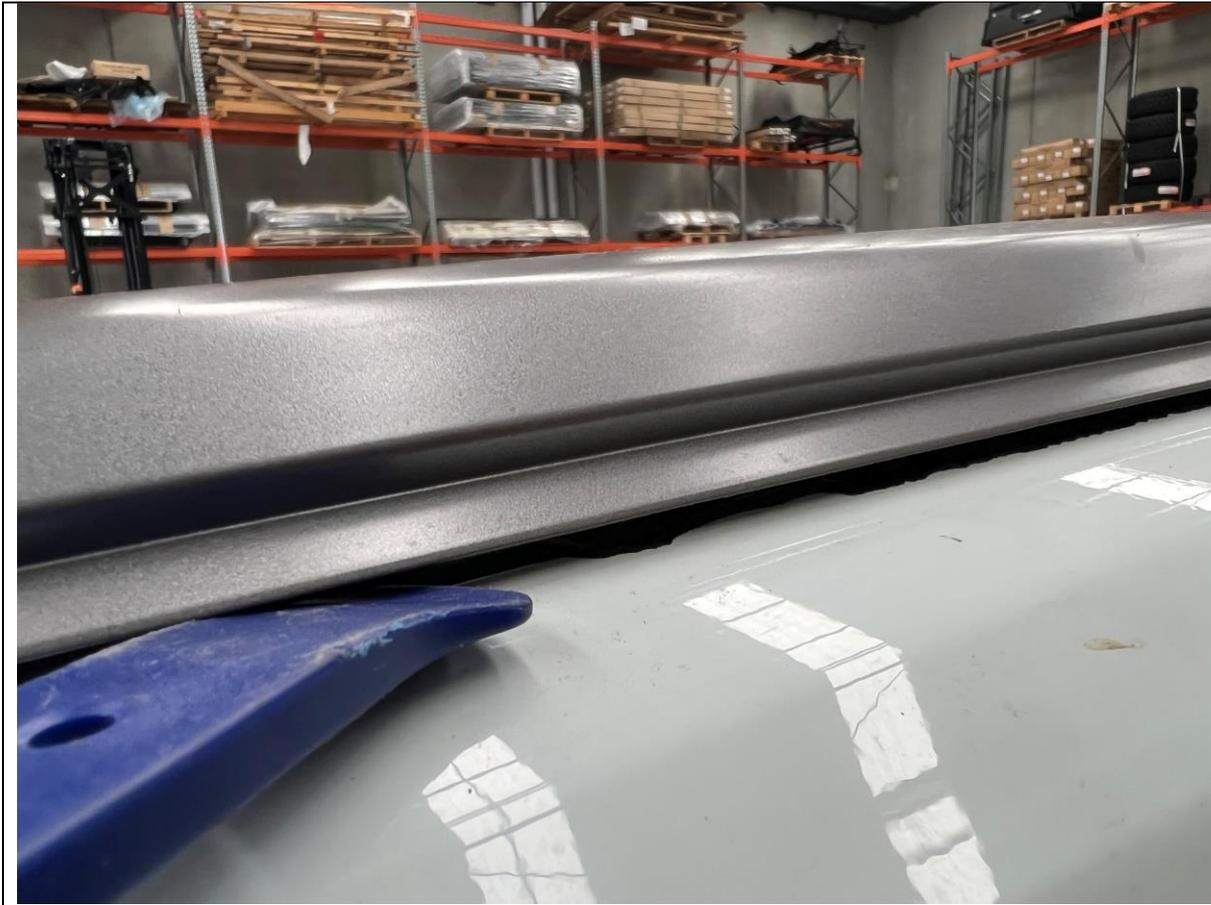
13. Working from one end, carefully pry the roof rail off the roof surface, gradually releasing the adhesive strip as you go.
