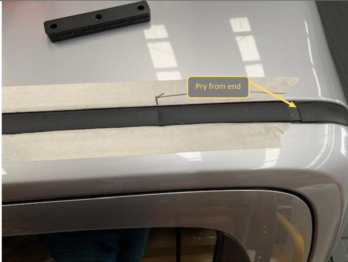
1. Place masking tape on the roof adjacent to the rubber roof trim.
