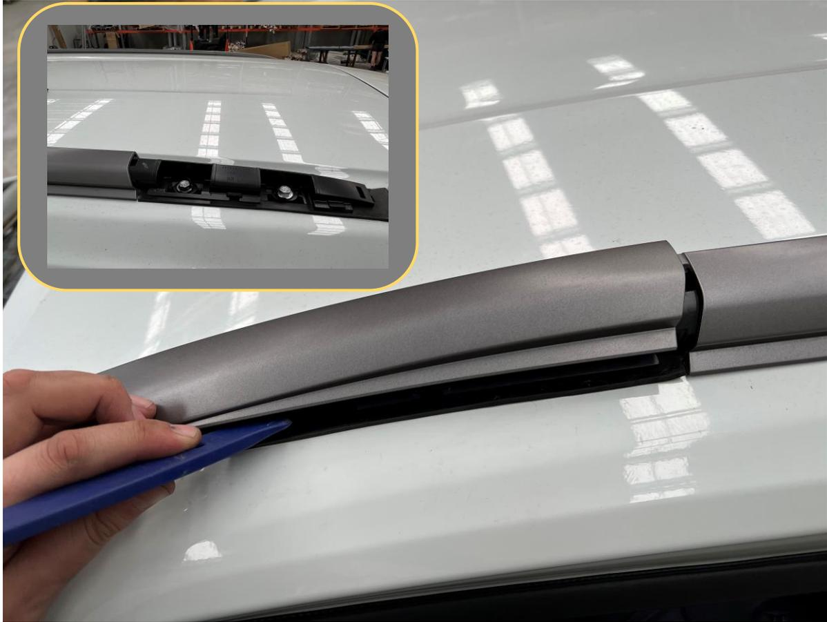
8. Using a plastic trim tool to prevent marking of roof, unclip the plastic cover at the front end of the roof rail, uncovering the forward roof rail bolts
