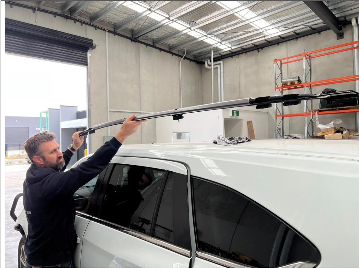
14. Once adhesive is released, lift off factory roof rail.
