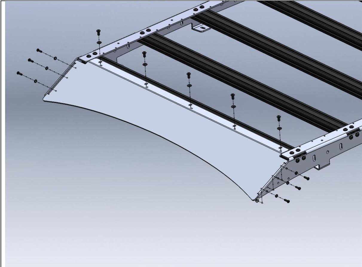
28. Secure the wind deflector to the side rails with M6x16 button head bolts, Flat washers, and flange nuts.
