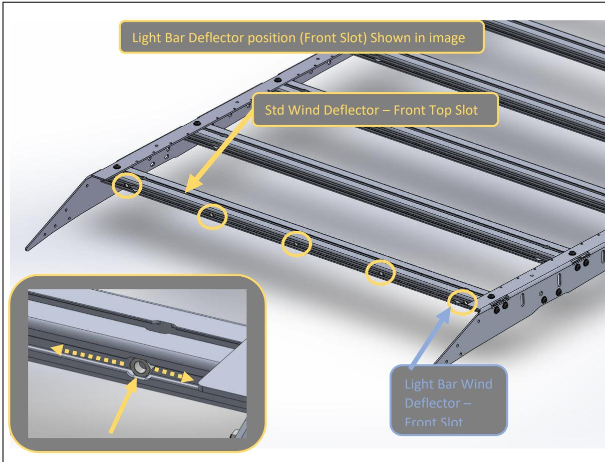
24. If fitting the standard wind deflector fit the 5x M8 nuts to the top front slot of the front most extrusion member.
