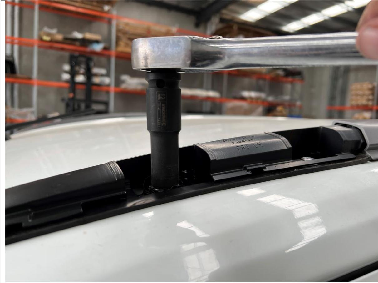
11. Remove the front and rear track bolts, using 12mm socket or spanner.
