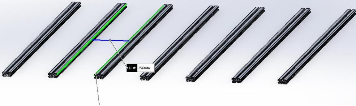
16. Next Assemble the roof rack. Start by setting out the 7 extrusions on a table. Position them so they sit approximately 250mm apart.
