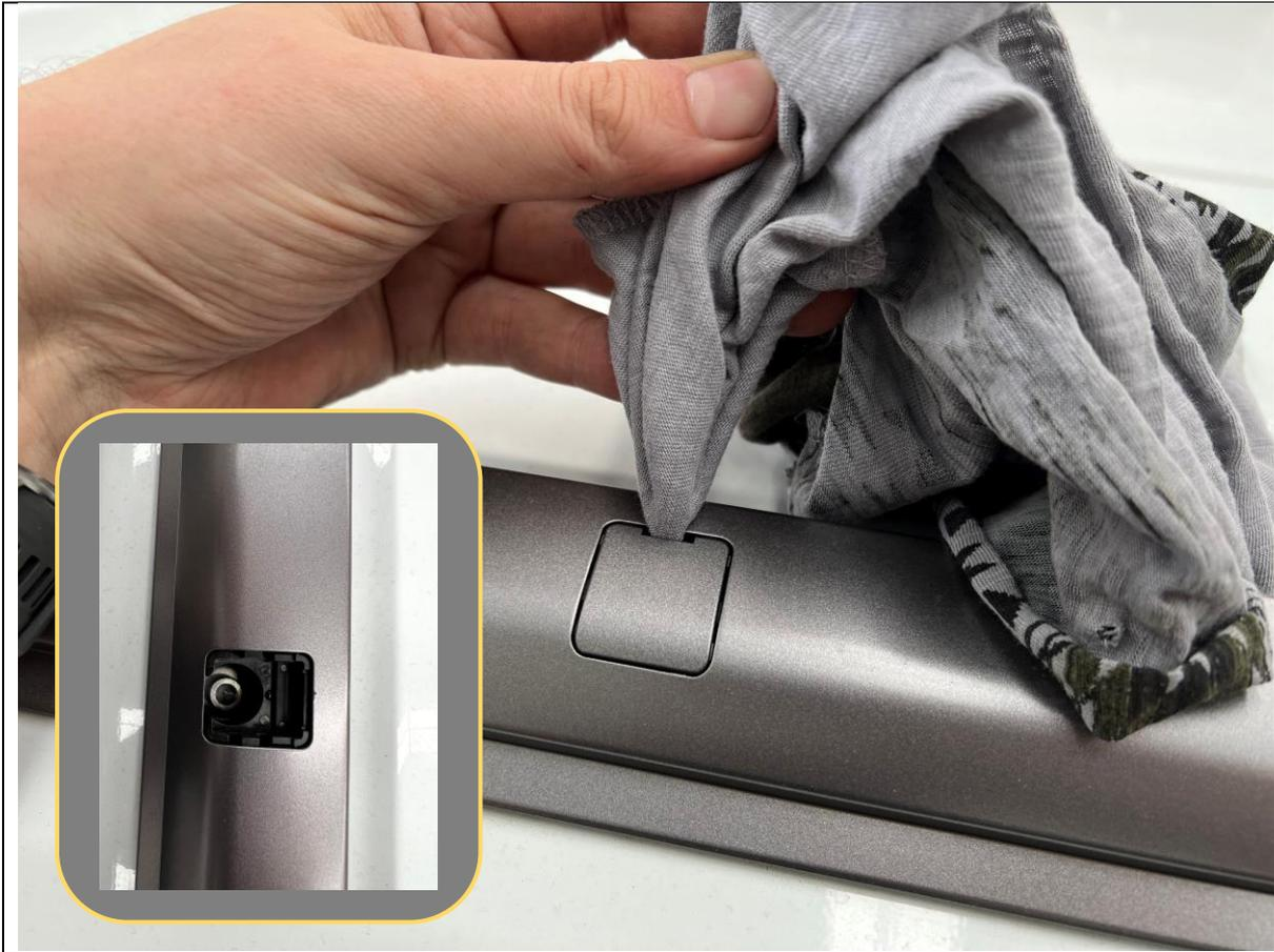
9. Using a Rag covered flat screwdriver to prevent marking of roof rail, unclip the plastic access covers at for the two center roof rail mounts, uncovering the forward center rail bolts
