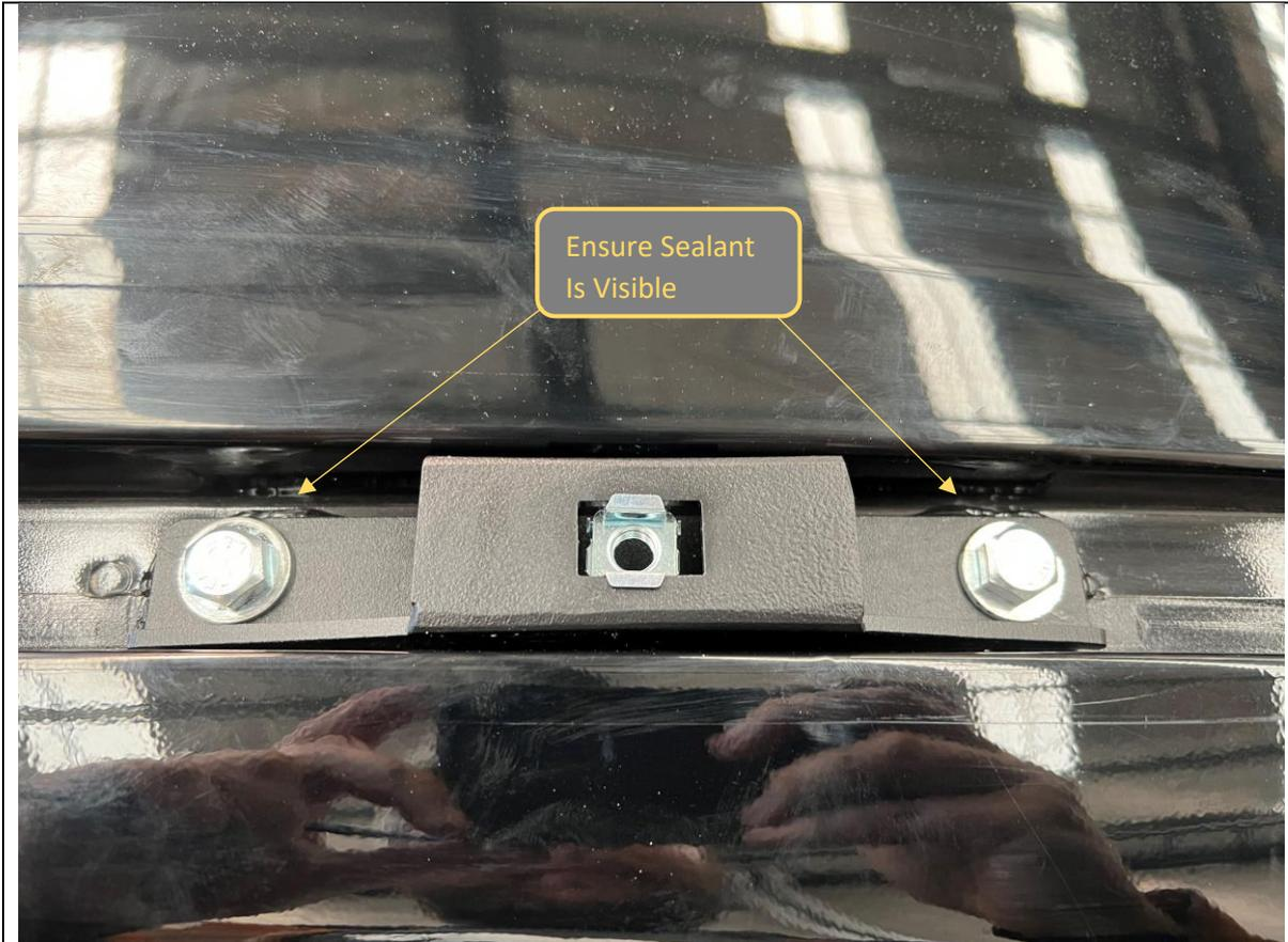
43. After mounts are tightened check sealant. Squeeze out should be visible around all mounts.
