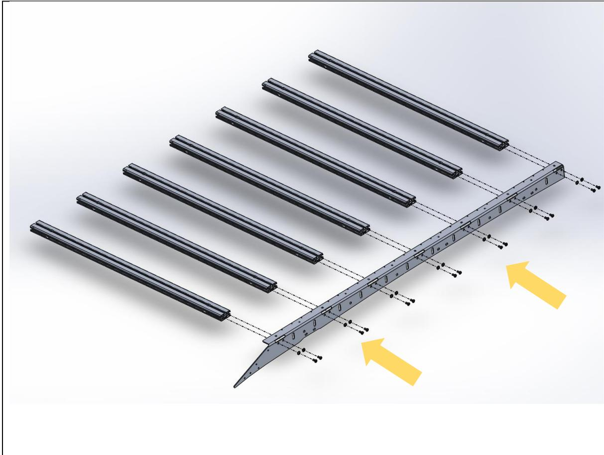
17. Fit the side rail to the extrusion,
