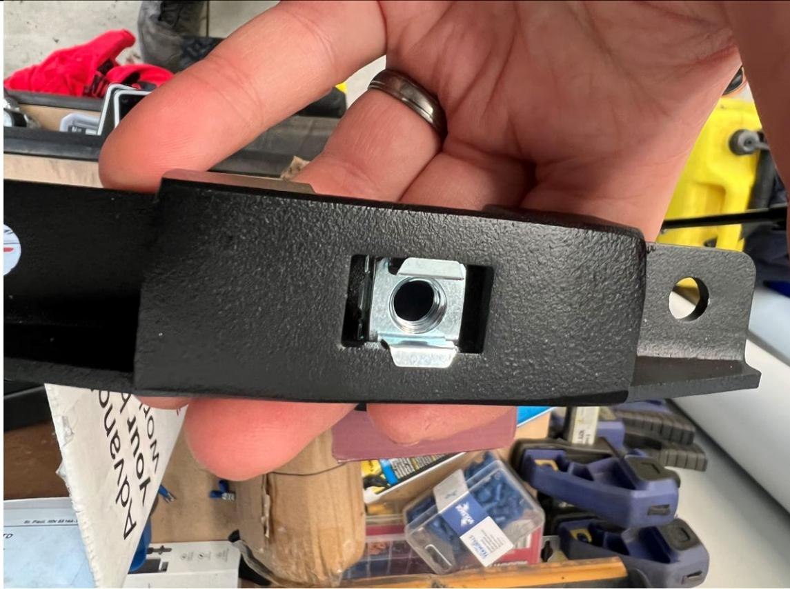
31. Pre fit the M8 Cage nut to the front and rear mounting brackets. A small flat screwdriver can be used to assist in pushing the cage nut into position.
