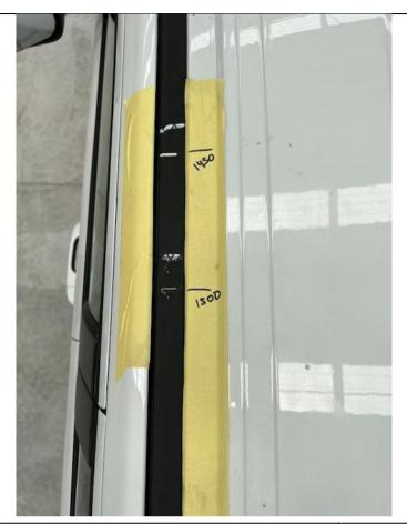
5. Mark the next lines going forward at 1300mm and 1450mm.
