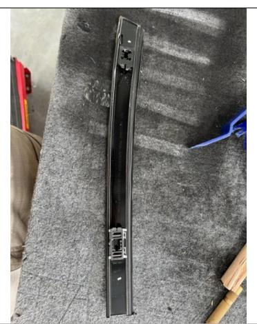
9. Section of the trim to be reinstalled, with keepers in place
