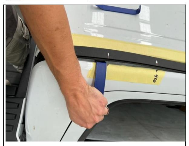
6. Using a plastic trim tool or rag with a flat head screw driver (take care not to scratch the roof paint) pry up the trim section all the way along
