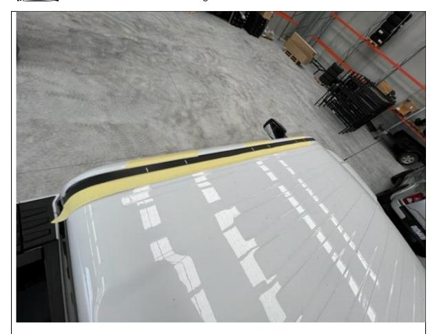
1. Place Masking tape on the roof either side of the gutter trim pieces.
