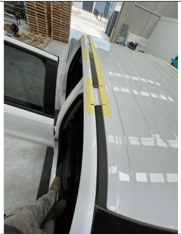
10. Refit the trim as shown leaving the marked sections bare
