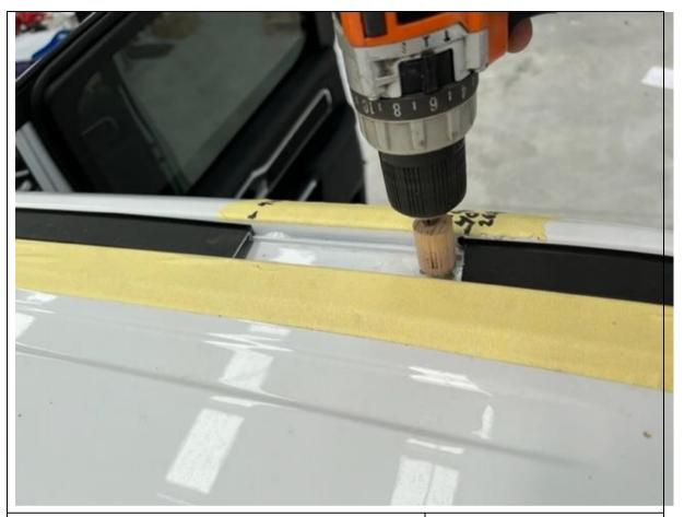
16. Drill the roof out to 11mm. Start with a pilot drill of 5mm. Ensure nutsert fits in each hole, you may need to drill through 2 layers of steel.
