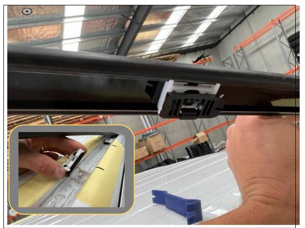
7. Remove keeper pieces from roof and refit on to the trim section.
