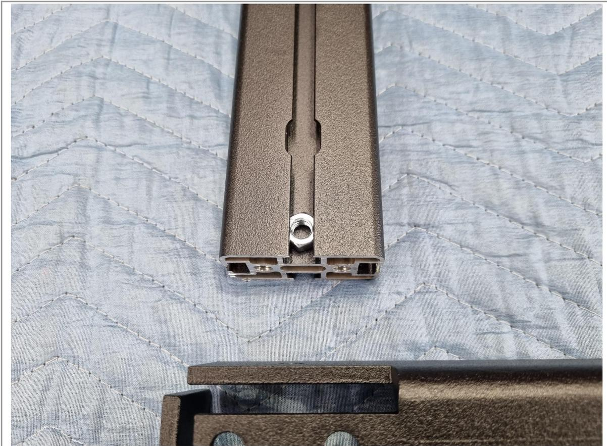
2. Insert 1x M8 nut into the top T-slot of the extrusion end.
