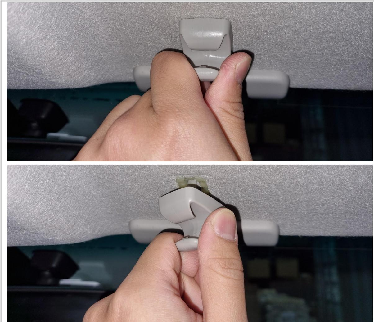
23. Grab onto the sun visor retaining clip and twist to release from the roof. (Twist anti-clockwise for the RH driver side, clockwise for LH passenger side)
