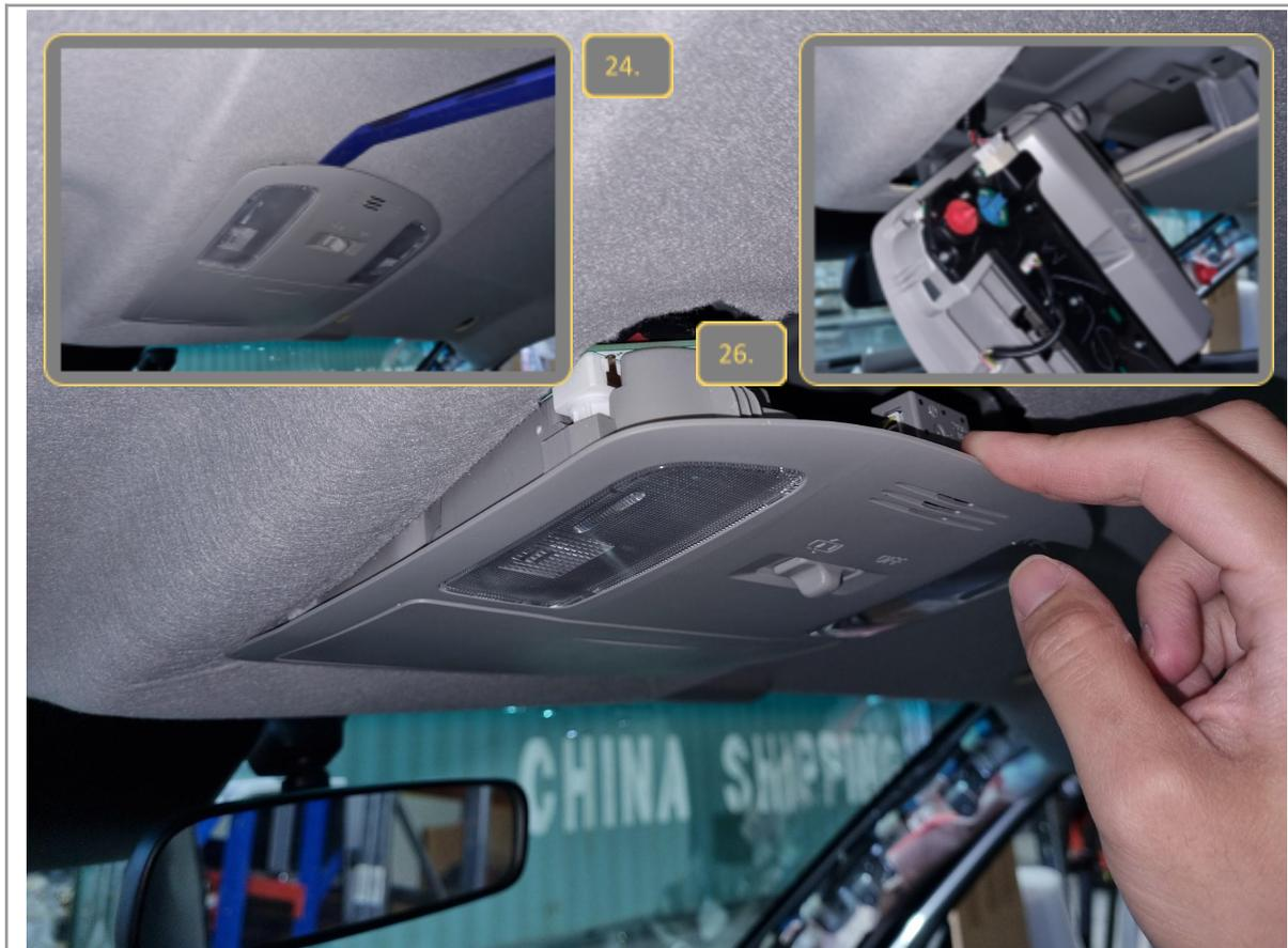
**FRONT OVERHEAD LIGHT CONSOLE REMOVAL**
