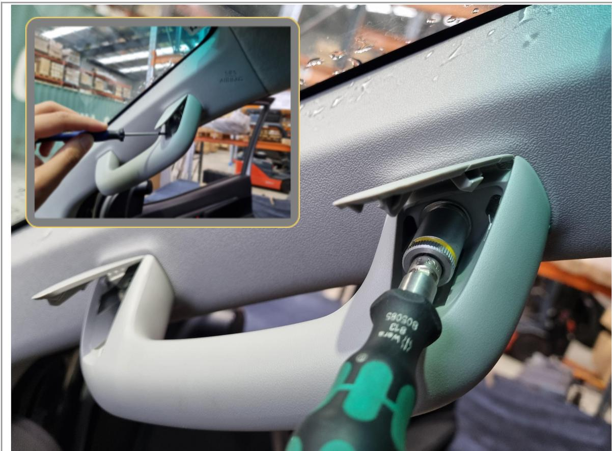
15. Headliner removal is required for fitting the roof rack. Start from the front and work your way backwards.
