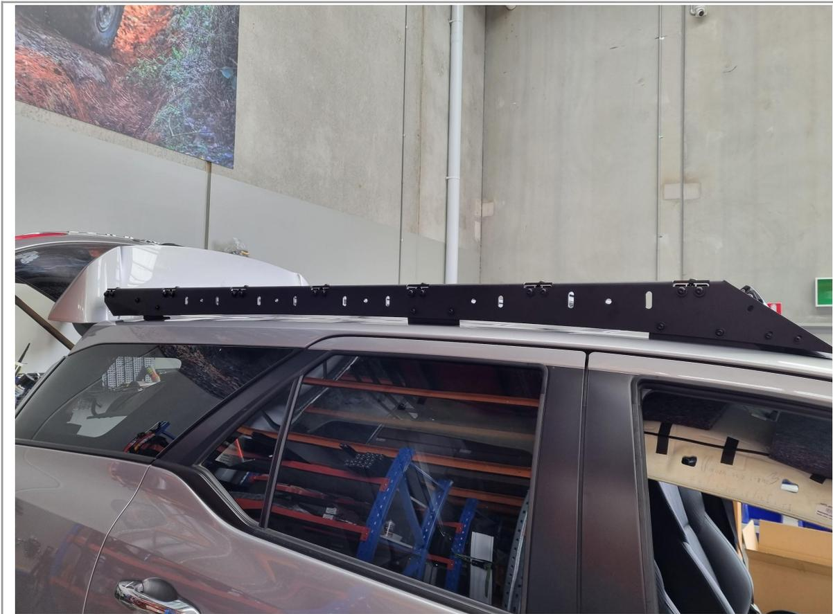
71. Adjust the roof rack so that there is 10-15mm of vertical clearance to the roof all the way around. Do the same for the wind deflector at the front.
