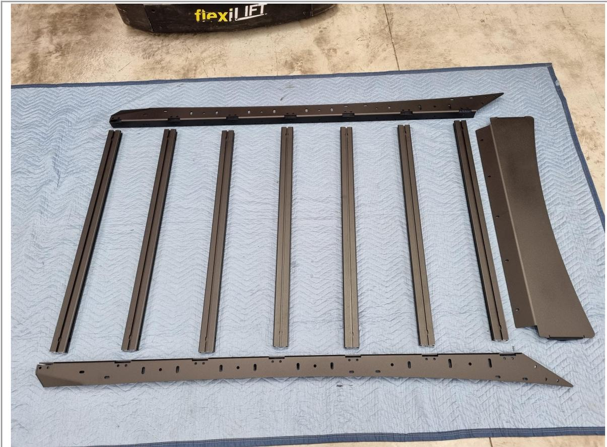
1. Find a large table space or floor area and lay out all of the extrusion cross bars, rack sides and wind deflector of choice.
