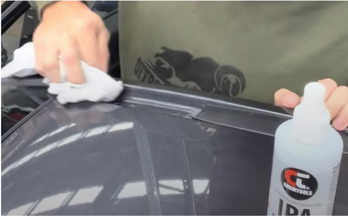
57. Using a cleaning solvent like isopropyl alcohol, give the roof channel a good clean. Make sure there is no dirt or oils left in the channel.
