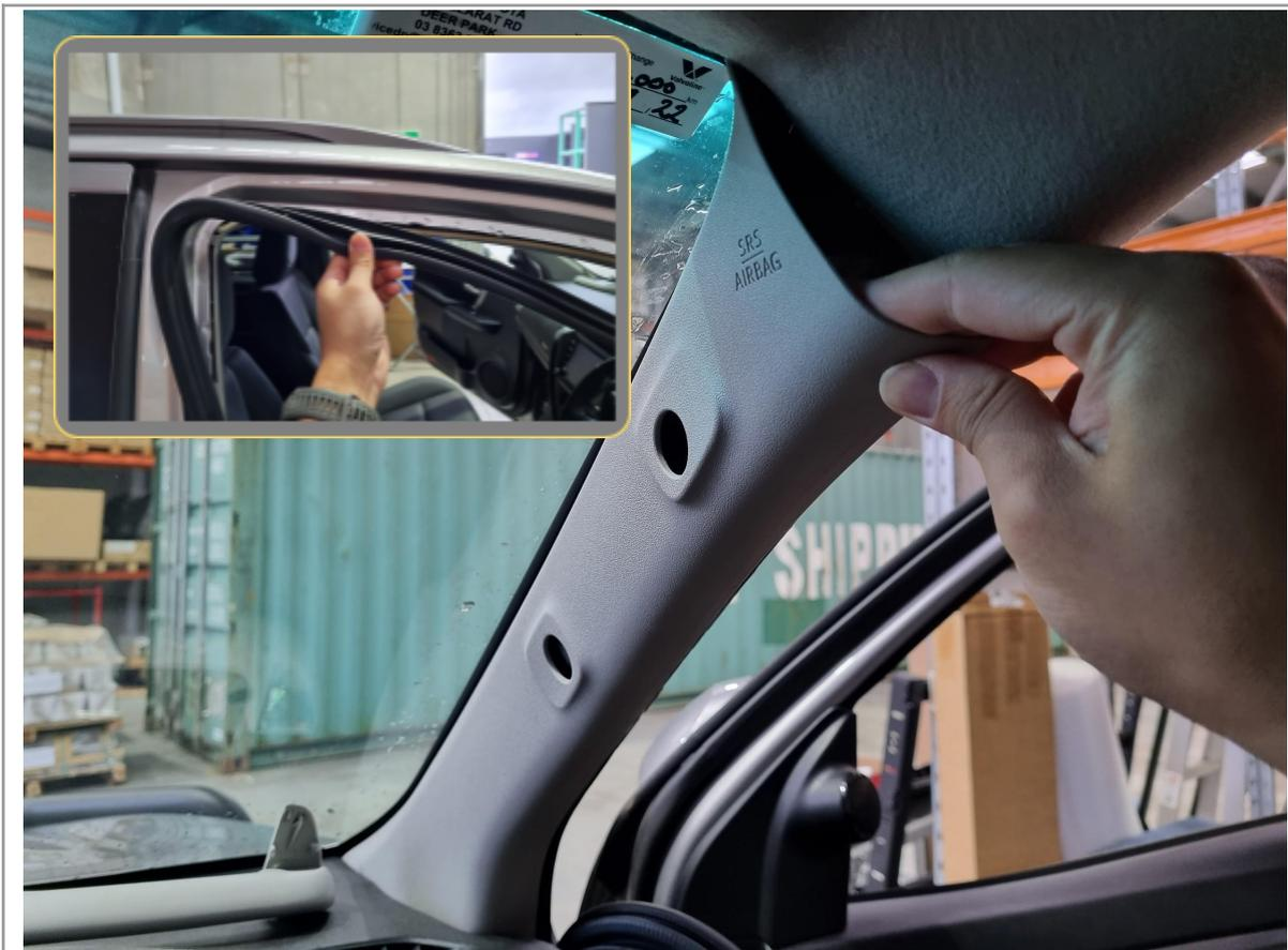
18. Pull back the rubber front door seal halfway to expose the A and B pillar trims.
