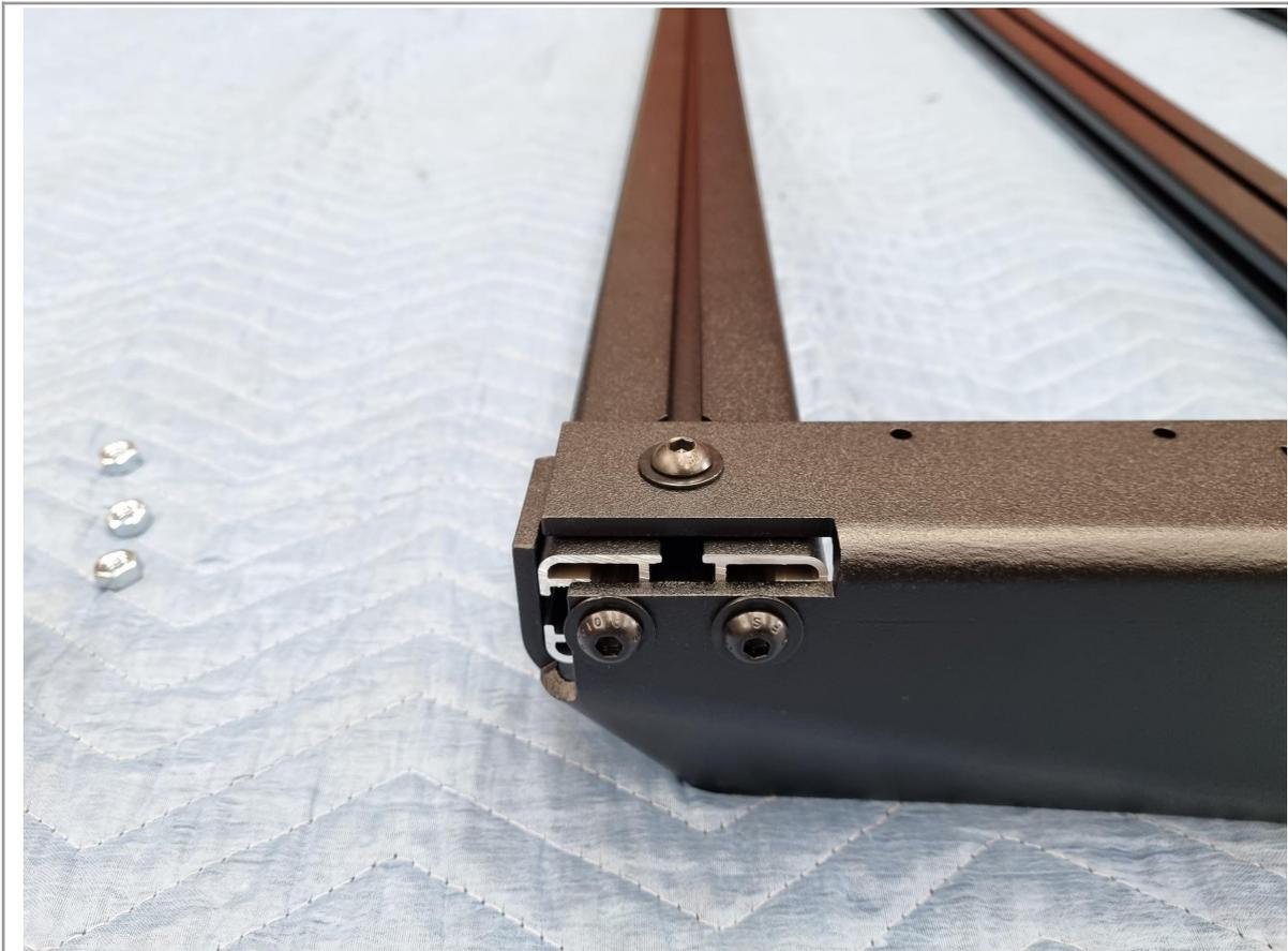
4. Bring the rack side in line with the extrusion and secure with 2x M8x20 button head bolts and black washers through the pre-threaded holes on the side and 1x M8x16 button head bolt and black washer through the previously installed M8 nut on top. Do not fully tighten.
