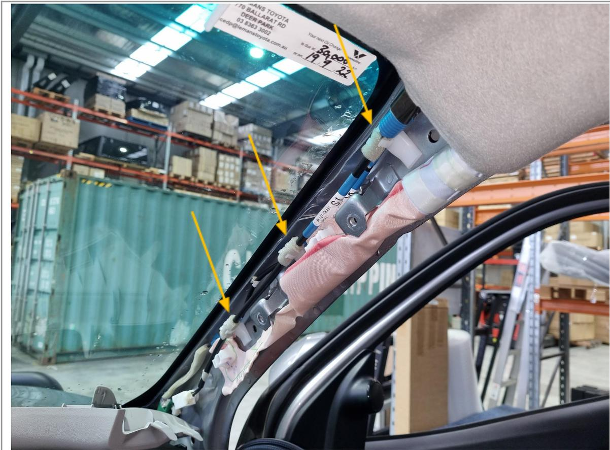
20. Carefully unclip the exposed curtain SRS airbag wire from its plastic clips as indicated.
