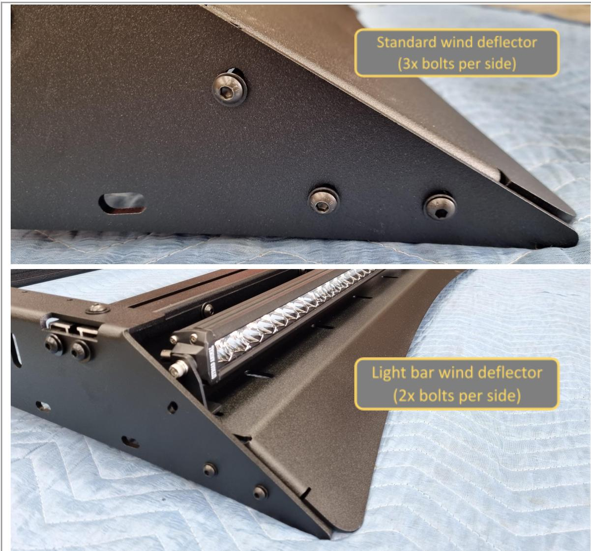
10. Secure your wind deflector to the rack sides with M6x20 button head bolts, washers and flange nuts.
