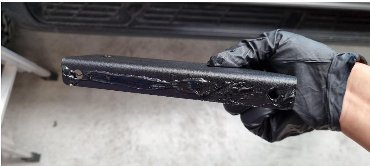
58. Starting at the front RHS of the vehicle, spread a good quality silicone adhesive sealant around the mounting holes in the roof channel.
