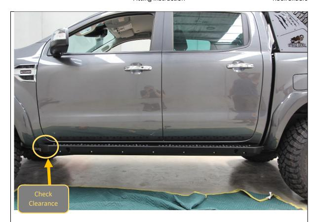
34. Adjust fore / aft position of sliders on mounts to achieve even appearance if required.
