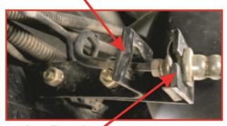
Top hole in bracket aligned with bottom mount bolt in chassis rail
