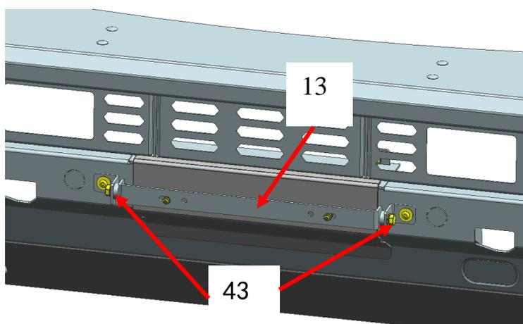
Step 9 Test and make sure that the guard is steadily fixed and fully tighten all hardware.
