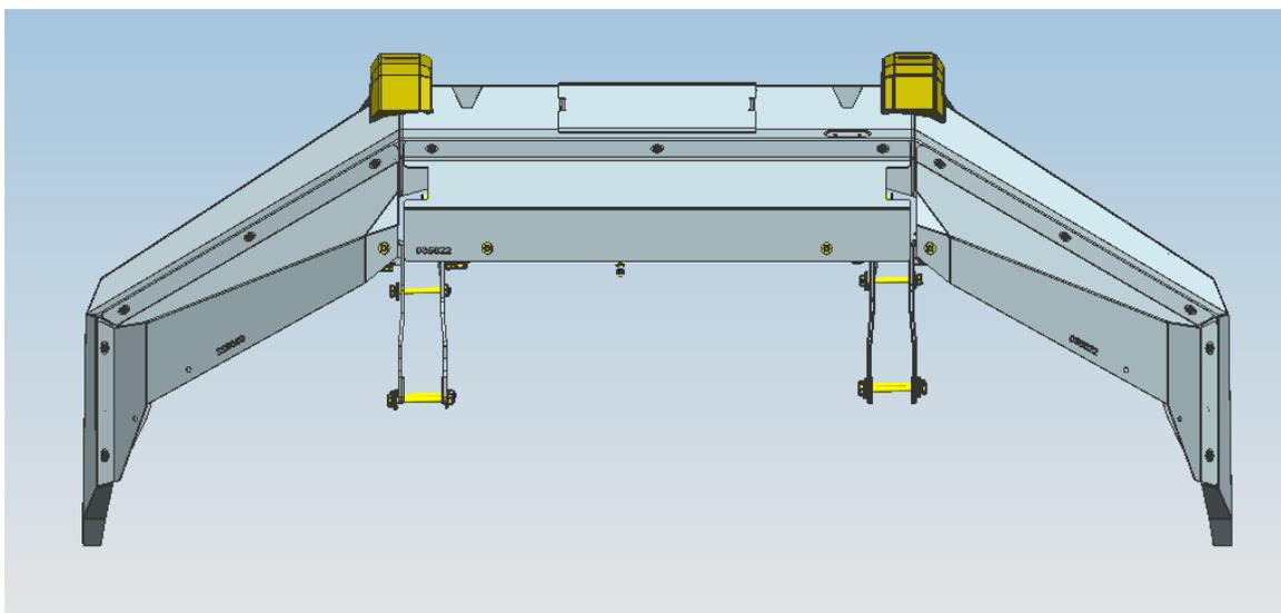
Step 9: Install factory bash plate by using factory hardware and supplied brackets.
