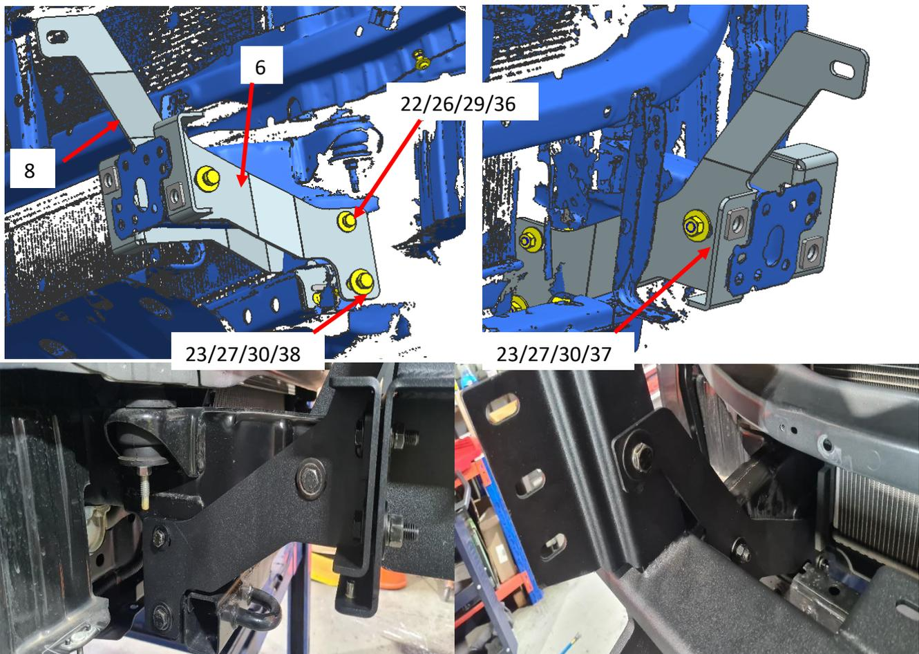
Step 5: Install the winch frame with hardware shown below.
