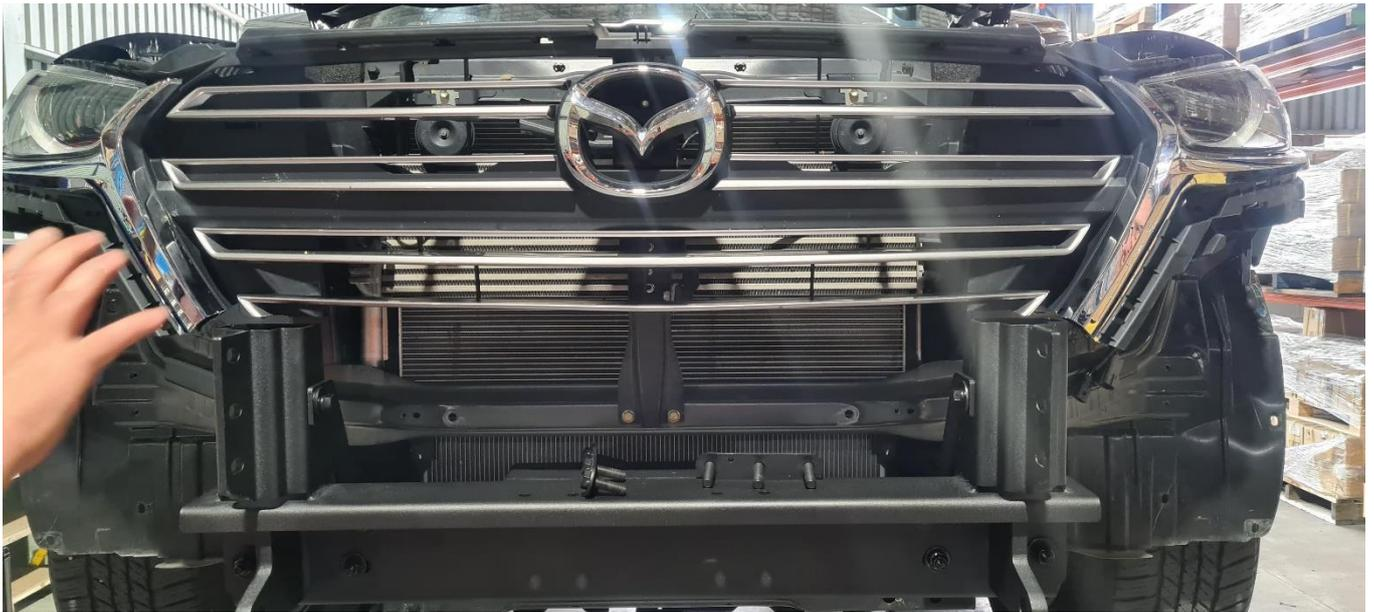
Step 7: Install the bull bar main body with hardware shown below
