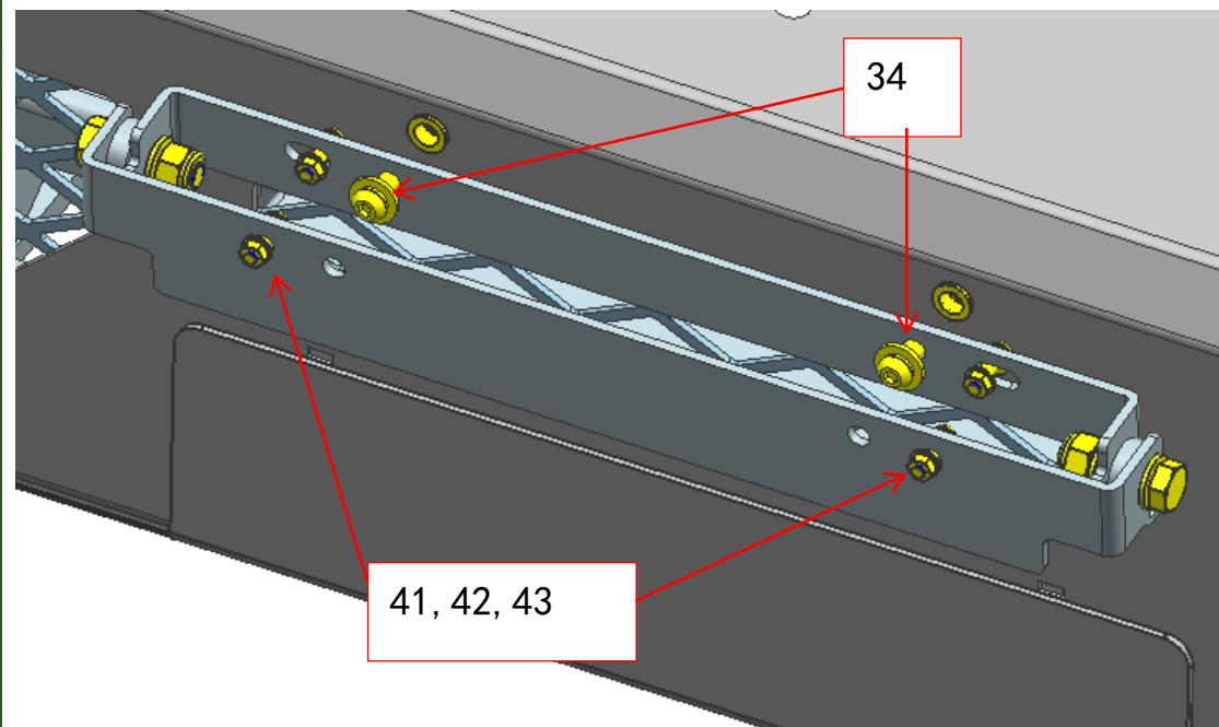
41 Cross cup head bolt M4\_16 42 Hex Nut M4 43 Flat Washer D4 34 Inner hex flat head bolt, spring washer and flat washer assembly M6\_20
