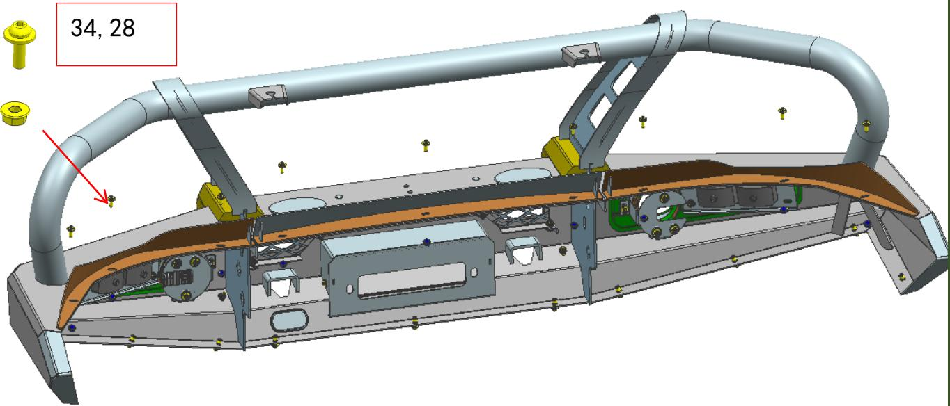
2. Connect the main bull bar assembly and winch frame after installing the three side wing bodies. Then adjust the distance between side wing bodies and vehicle to 15-20mm, the distance between side wing bodies and mid connection to about 6mm, and then tighten all hardware.
