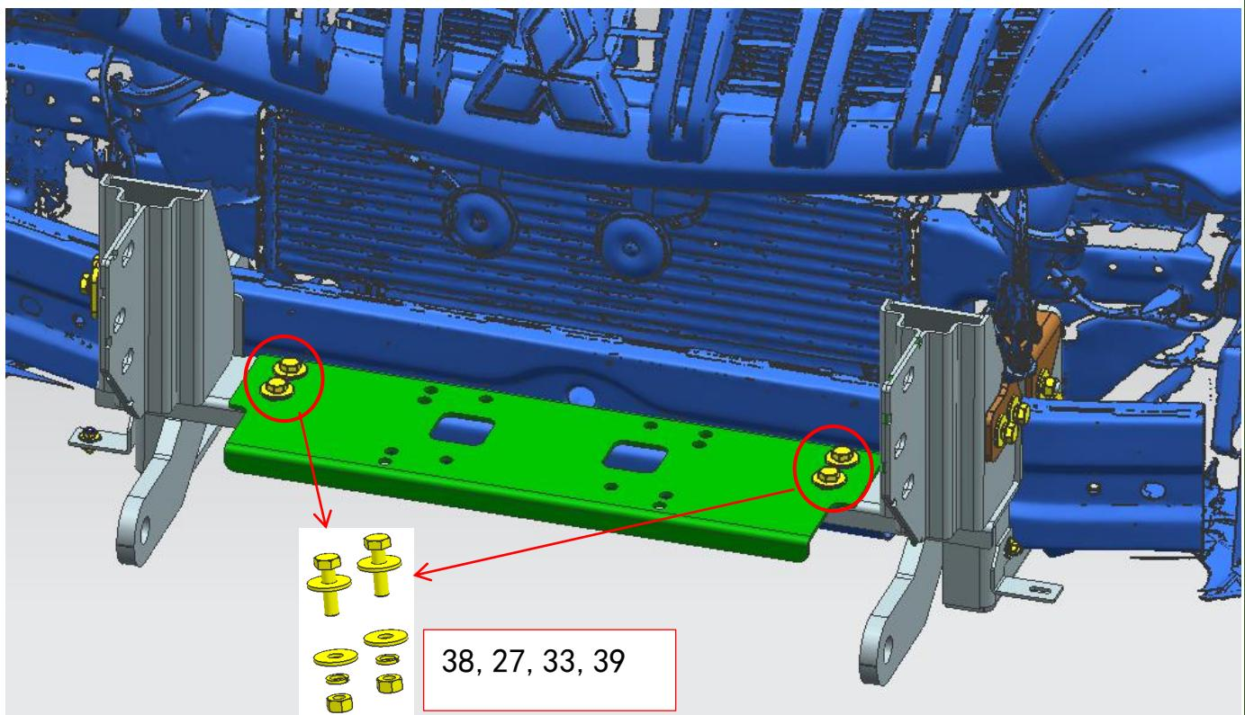
3、Adjust the center distance of winch frame and keep it between  $730\pm2\text{mm}$ . Then tighten all hardware. Connect support bracket 2 with winch frame and tighten as below picture.
