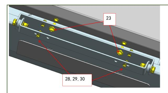
Step8: Test and make sure that the guard is steadily fixed, fully tighten all hardware.
