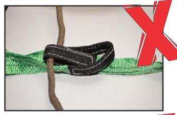
This method is one of the 'downright dangerous' options - bascially the end of strap A is insterted through the eye of strap B and a stick inserted through the eye of strap A. All the force in the recovery is going through the stick. The problem here is if (when!) the stick breaks or the straps let go, there is nothing to hold the straps together, and they will recoil with tremendous force.
