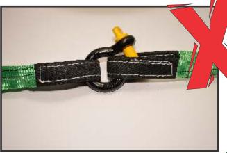
This method is another of the 'downright dangerous' options - joining strap A & B with a chackle. NEVER use a shackle to join straps. If the strap breaks, the unbroken strap and shackle will recoil with enough force to cut down anything in its way.
