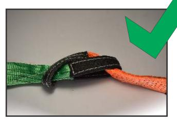
This method is pretty much a standard REEF Knot. The eye of strap A is passed through the eye of strap B. Then the other end of strap B is passed through the eye of strap A. This produces a strong join. The downside is that this joint will be extremely difficult (sometimes impossible) to undo after use.
