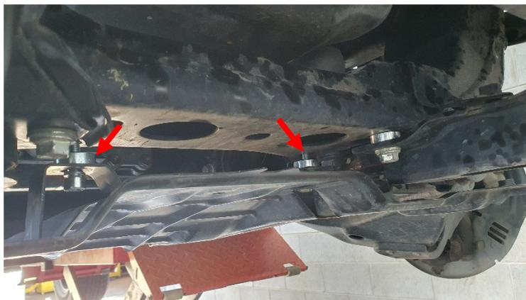
9. Reinstall the bash plates using the OEM hardware.
