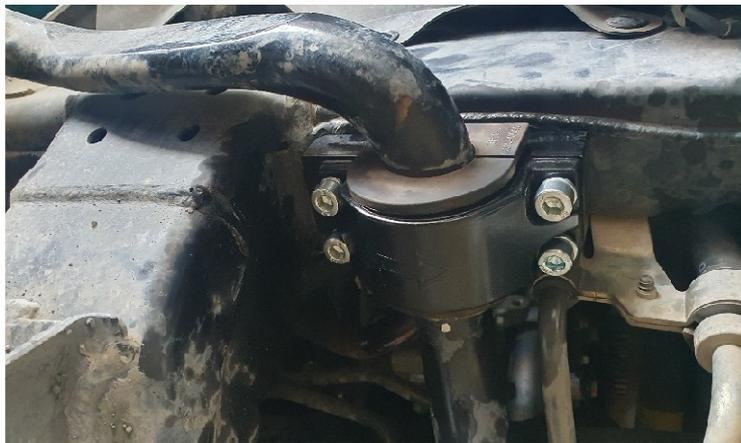
7. **NOTE:** If installing a diff drop kit as well, this will typically be supplied with slightly longer bash plate spacers to allow clearance of the lower diff position. If this is the case use those spacers and bolts supplied instead and skip the remaining steps.
