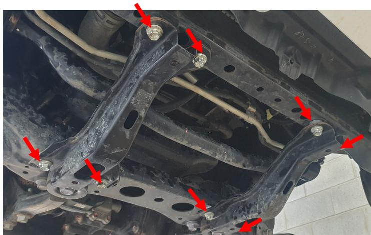
8. Install the 8mm spacers below the front of the under diff bash plate and use the M8 bolts supplied with washers and spring washers.
