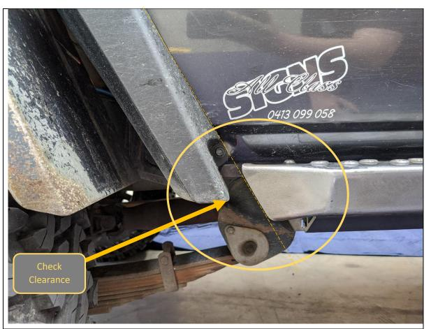
36. Adjust fore / aft position of sliders on mounts to achieve even appearance if required.
