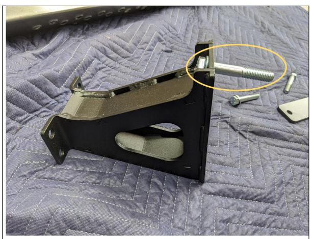
15. Prepare mid and rear mounts for fitting by threading throught M12x90 Bolt through top hole.
