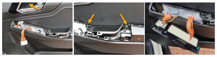
· Position the window switch fascia front end first so it engages the locating lug and lower back into place
