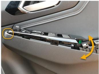
The switch fascia assembly can now be pulled out and turned upside down to gain access to the two connectors
