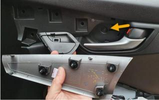
• The two (larger) Phillip's screws from under the armrest and switch fascia for all models can be removed
