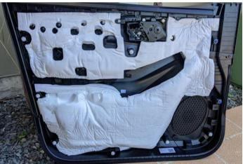
• The door card can now be put aside, if any plastic clips have remained in the door panel remove them now and place back into their respective positions on the door card.
