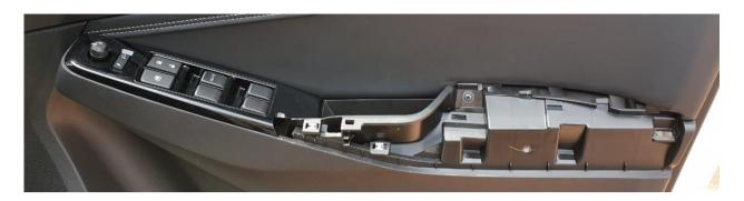
• Remove any clips left in the door panel and place them back into position on the armrest.
