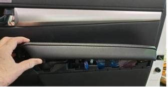
Before the padded armrest can be completely removed you will need to lift the white retaining clip by pressing it upwards
