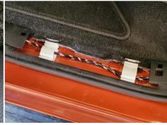
Pull off the rubber door seal on the right-hand side
