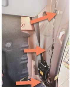
• Remove the existing factory rubber grommet by compressing the edges and pushing it inwards, out the back of the cab (this will not be reused)
