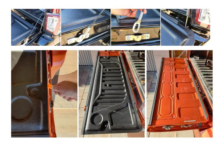
Remove the remainder Phillips screws, the metal cover can now be removed.
