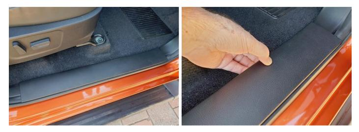
The kick panel also needs to be removed, first undo the small plastic nut and then dislodge the single retaining clip.
