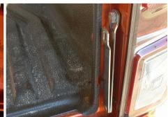
For MY23 models that have factory fitted easy up/down struts, remove one of the wire ends supports, the struts are <u>not required</u> to be removed.
