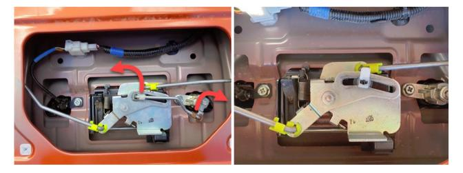
**NOTE:** Do not operate the latch assembly until the replacement connecting rod is fitted, operating may deform the plastic clip and dislodge the thin plastic washer located on the underside.
