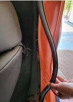
• Dislodge the trim, its clipped in place around the seat belt (it does not need to be completely removed just enough for the side trim to be taken out from underneath it
