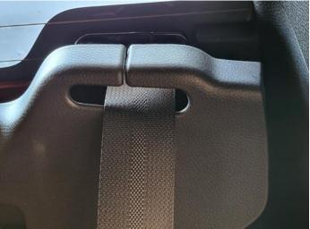
Remove the large side plastic trim by dislodging the clips, starting at the top
