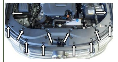
Remove rubber seal before removing plastic cover
