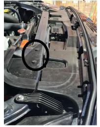
Remove the screws and clips from the front nose cone and remove
