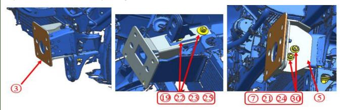
Step 4. Install Winch frame as below, including the skid plate connecting brackets.
